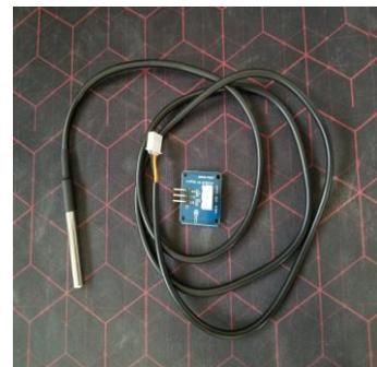
Fig. 3: Temperature Sensor
