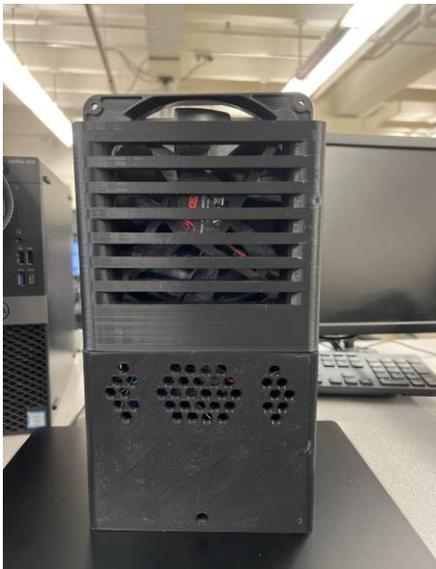
*Fig-1: Front View, consisting of the top half (air filter compartment) and the bottom half (air monitor compartment)*
