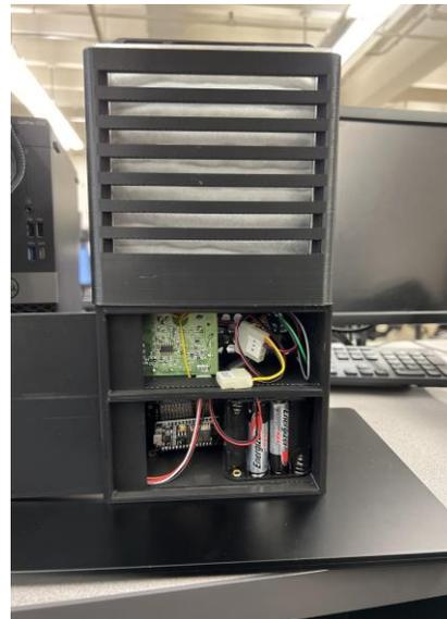
*Fig-2: Back View, revealing the battery compartment and circuitry*
