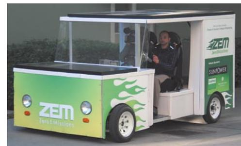
pedaling. The electric motor can power the vehicle to run at higher speeds, up to 35 mph. Solar energy provides a continuous charge of the batteries during the operation of the vehicle and also when it is idle. The vehicle has a cruising range of 40 miles. With the solar energy supplement, its range is 50 miles.
