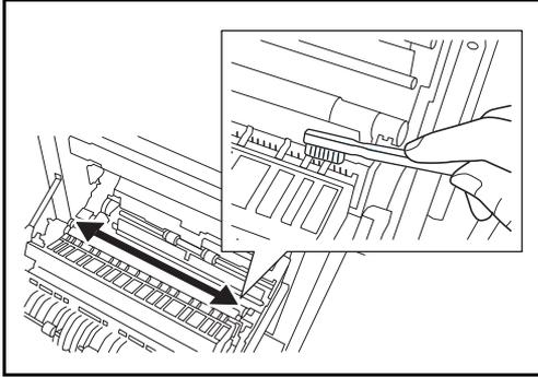
**15** As shown in the figure, clean dirt from the separator by moving the brush from side to side along the separator.
