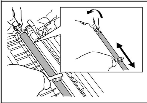
**16** As shown in the figure, clean dirt from the transfer roller by moving the brush from side to side along the roller while rotating the roller by turning the gear at the left end of the roller.
