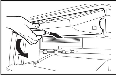
Adjust the angle of the operation panel in two as shown by releasing the operation panel lock lever.
