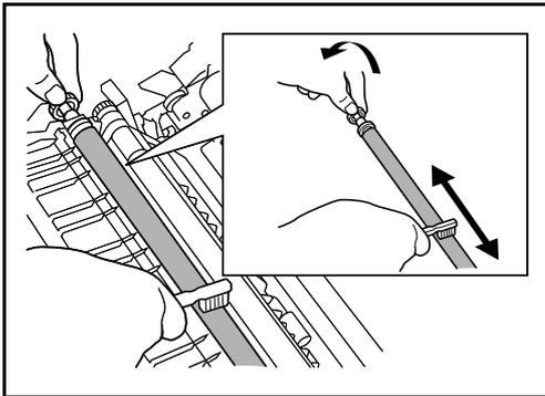
4 As shown in the figure, clean dirt from the transfer roller by moving the brush from side to side along the roller while rotating the roller by turning the gear at the left end of the roller.
