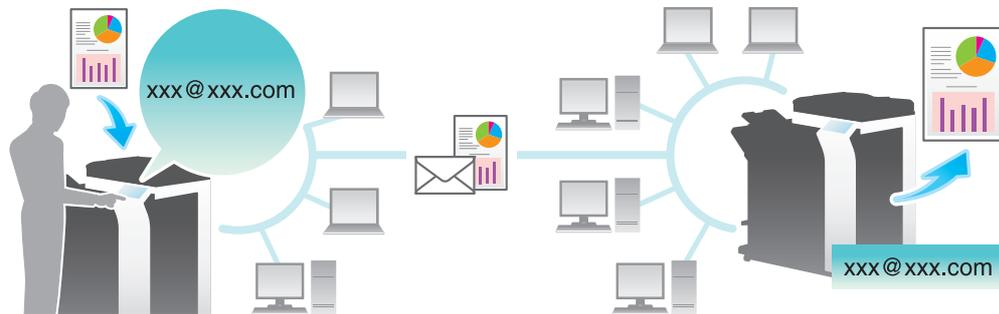
Within your intranet, the IP Address Fax function can be used. For IP Address Fax, specify either the IP address, host name or E-mail address of the destination fax machine to directly send a fax to that destination. No mail server is required.
