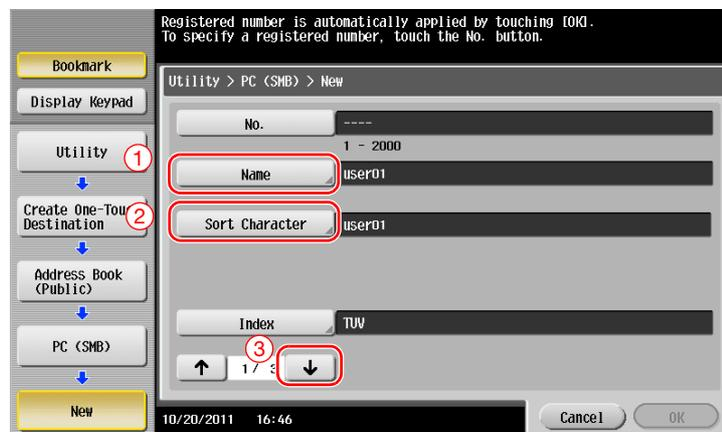
→ This sets the appropriate index for the name, which you entered into [Name], to [Index]. To change the setting, tap [Index].
