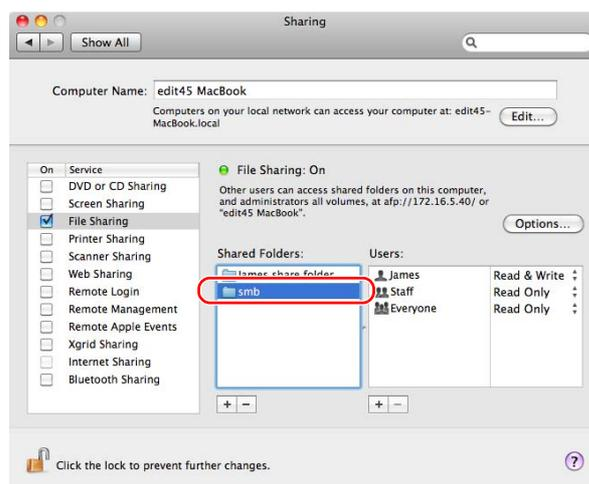
If the access right is changed to [Read & Write], the setting is completed.
