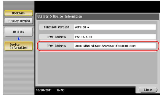
→ If no IP address is displayed, you need to configure the network. For details, refer to the User's Guide CD.
