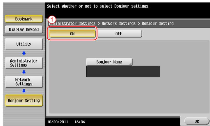
→ The Bonjour name is displayed on the printer driver as a connected device name. For "Bizhub C754 (5A:0C:4B)", "Bizhub C754" indicates the product name, and "(5A:0C:4B)" indicates the last three bytes of the MAC address.
