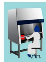
**If the fume hood fails:** Close sash to see if airflow improves. If flow does not promptly return, turn off heat and ignition sources. Close gas valves and chemicals. Close sash and evacuate the area. **GET HELP from safety staff.**
