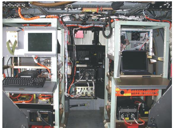
**Figure 2. Photograph of Army/NASA EH-60L cabin with air data system and research flight control computer console stations.**
