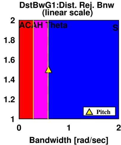
Figure 11. Pitch attitude disturbance rejection spec, ACAH
