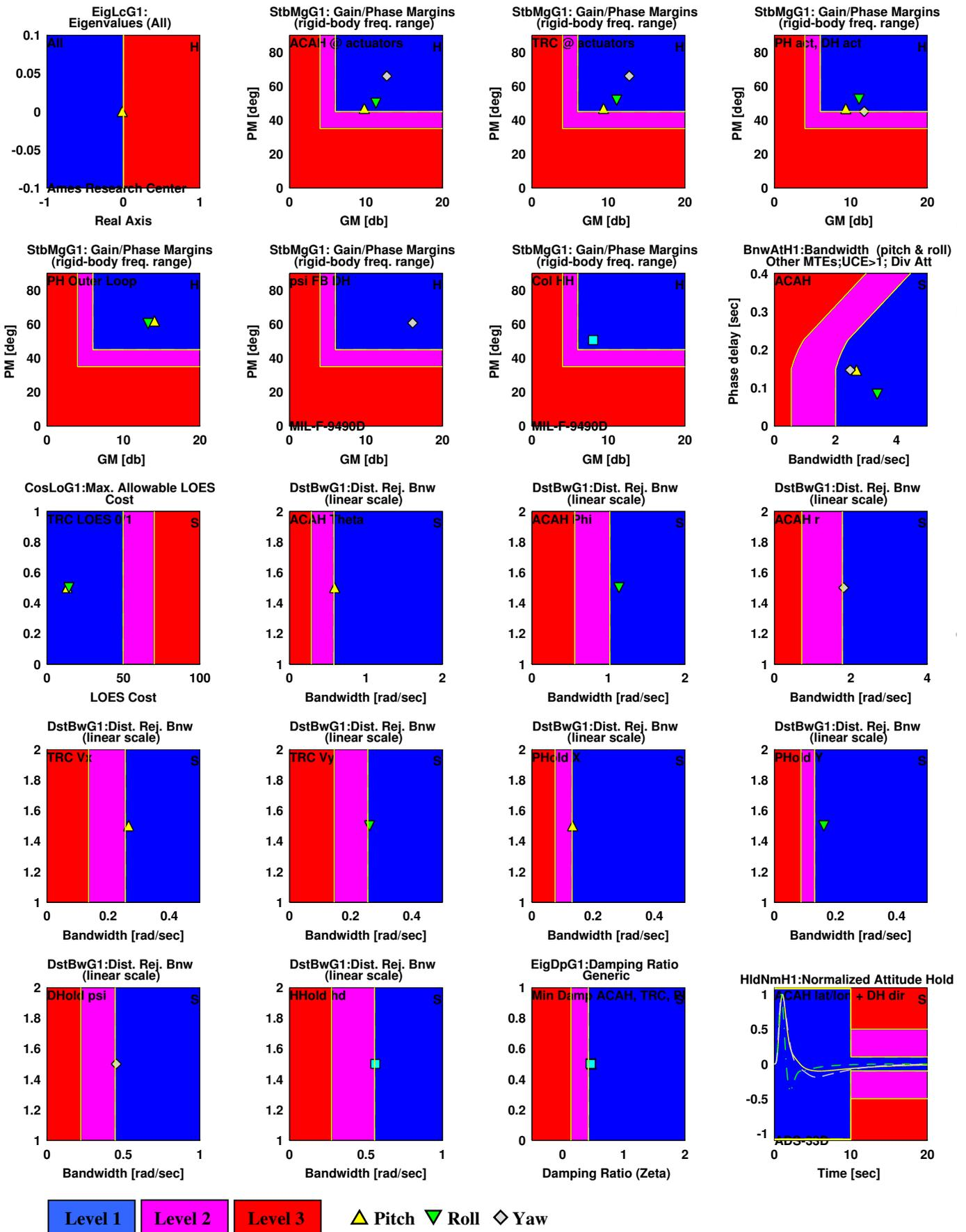
Figure 5. CONDUIT<sup>®</sup> Handling Qualities window (MCLAWS, partial)
