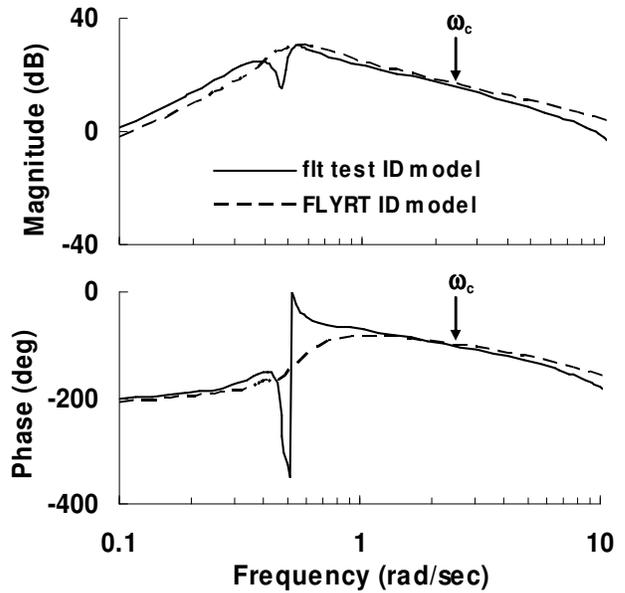
**Figure 2. Unaugmented pitch rate response comparison for identified linear models**
