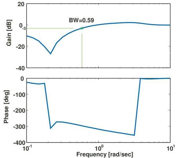
Figure 12. Pitch attitude disturbance rejection spec supporting plot, ACAH
