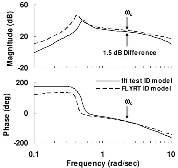
**Figure 3. Unaugmented roll rate response comparison for identified linear models**
