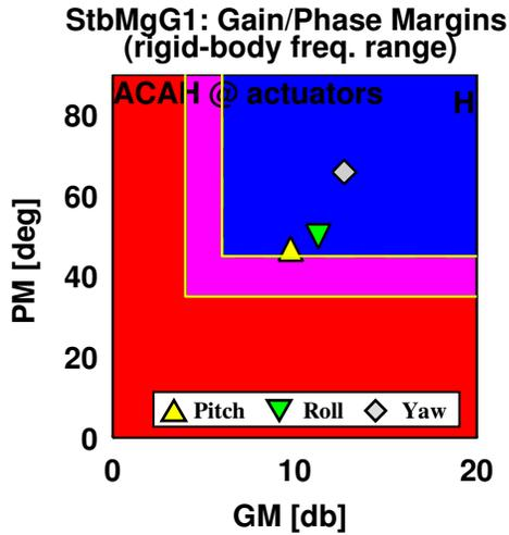
**Figure 6. Stability margin spec for pitch, ACAH, at primary actuators**
