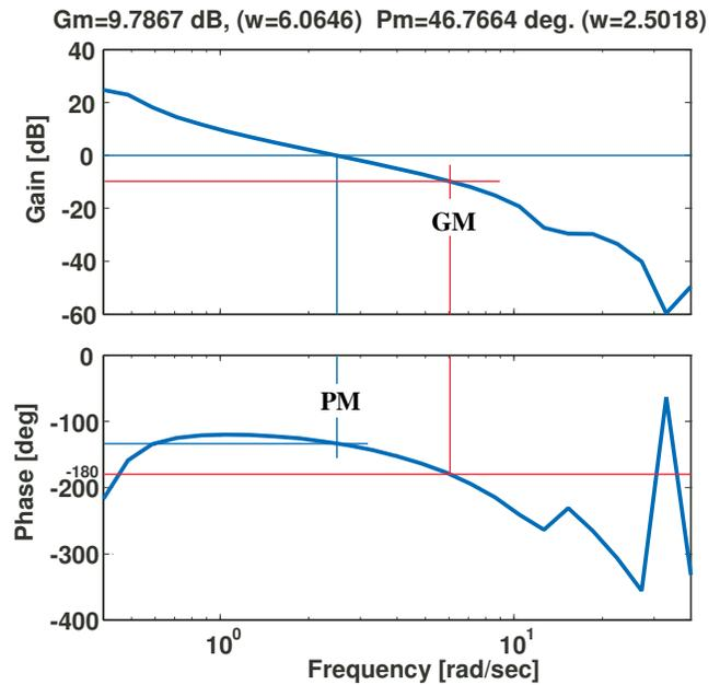
**Figure 7. Stability margin supporting plot for pitch, ACAH, at primary actuators**
