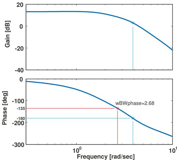
Figure 10. Bandwidth spec supporting plot for pitch, ACAH
