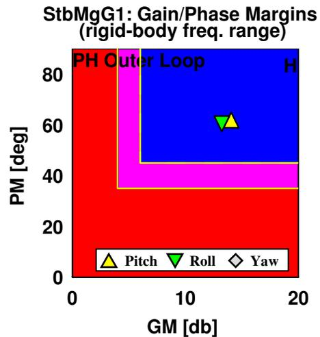
**Figure 8. Stability margin spec, PH, at outer loop position error calculation point**
