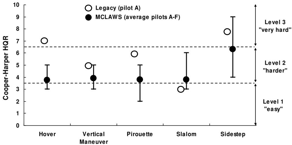
Figure 14. Handling qualities ratings from piloted simulation
