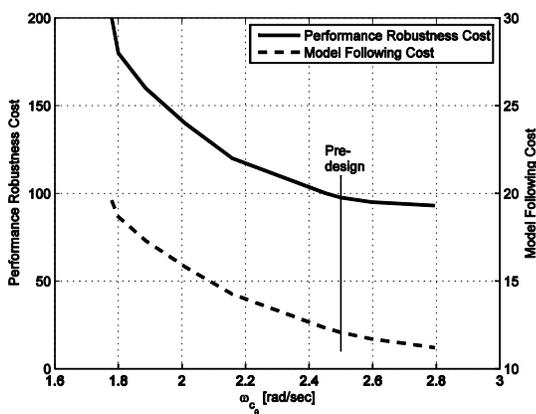
**Figure 8 – Variations in model following and performance robustness with changes in crossover frequency (from reference [12])**
