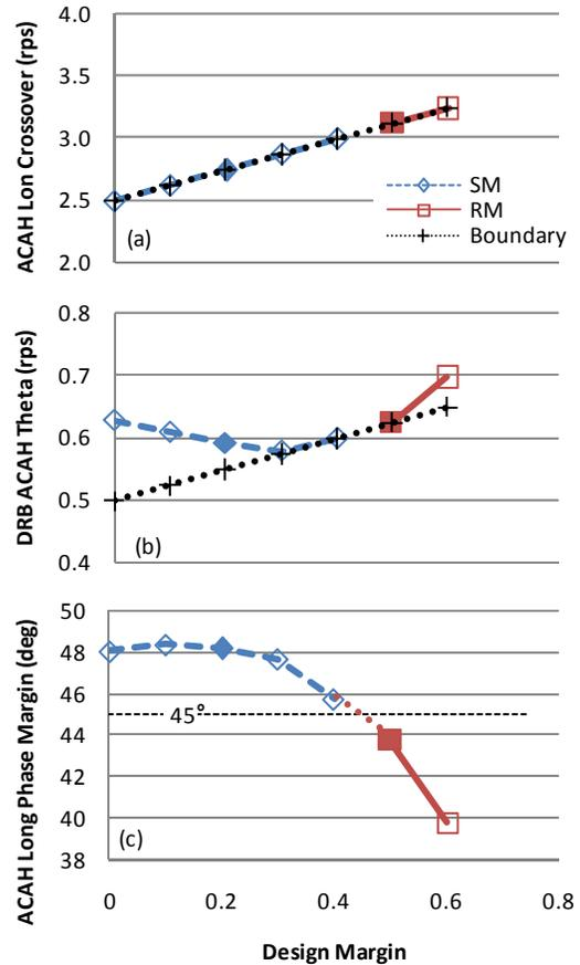
Figure 11 – Longitudinal inner loop results (flight cases filled)
