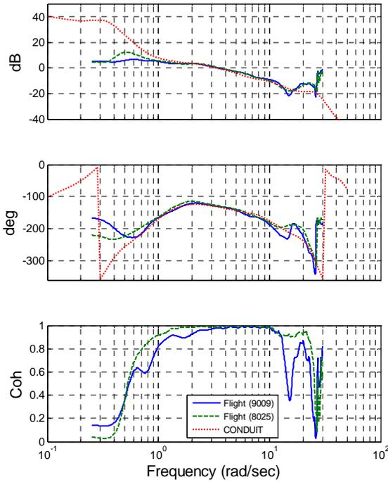
**Figure 3 – Longitudinal broken loop response comparison between analysis and flight**
