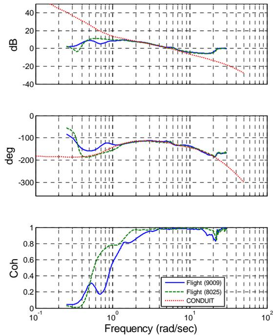
**Figure 5 – Directional broken loop response comparison between analysis and flight**
