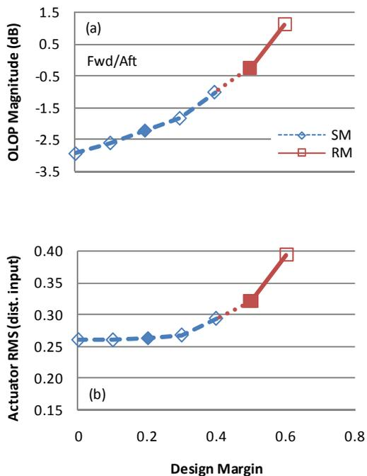
Figure 14 – Longitudinal OLOP and actuator RMS (for disturbance inputs) results (flight cases filled)
