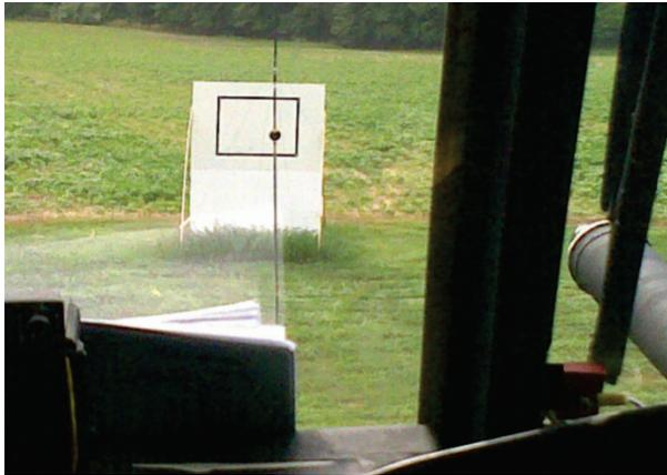
**Figure 23: Hover Board and Reference Symbol Used in Hover MTE**
