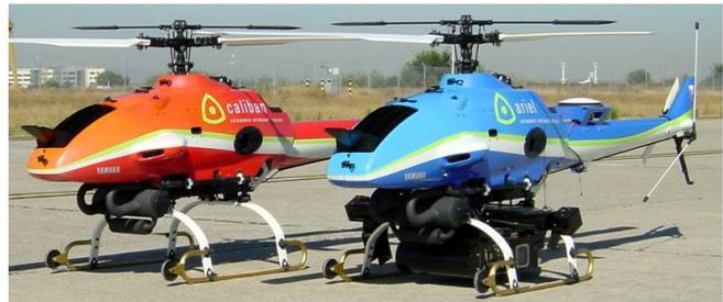
**Fig. 1. Autonomous R-MAX helicopters flown by the Autonomous Rotorcraft Project (ARP) at Moffett Field, CA**
