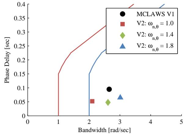
**Fig. 12: Bandwidths of the four pitch axis command model natural frequency configurations**
