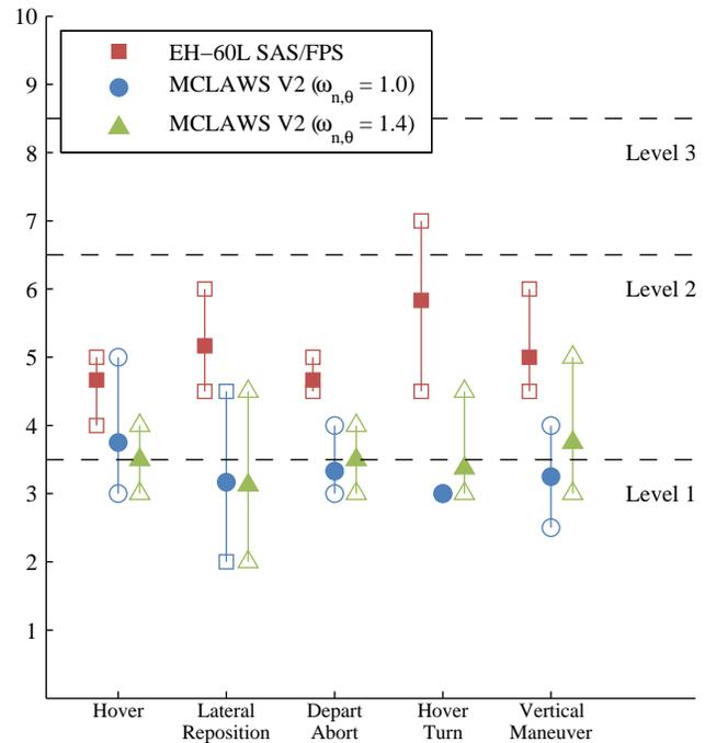
**Fig. 14: Comparison of handling qualities ratings for SAS/FPS and MCLAWS V2 in simulated UCE =2 conditions**
