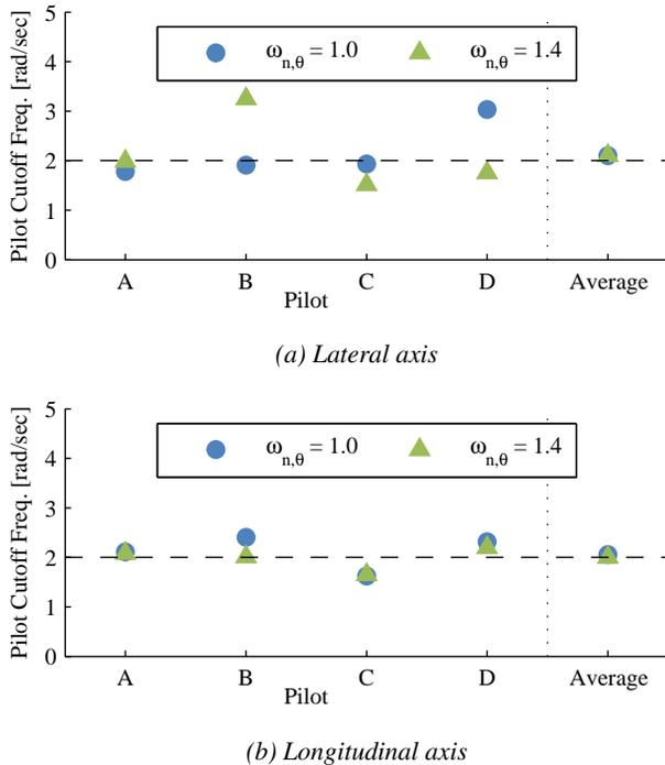
**Fig. 15: Average pilot cutoff frequencies for both MCLAWS V2 configurations**
