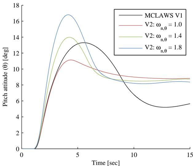
**Fig. 11: Pitch axis step responses of the four pitch axis command model natural frequency configurations**
