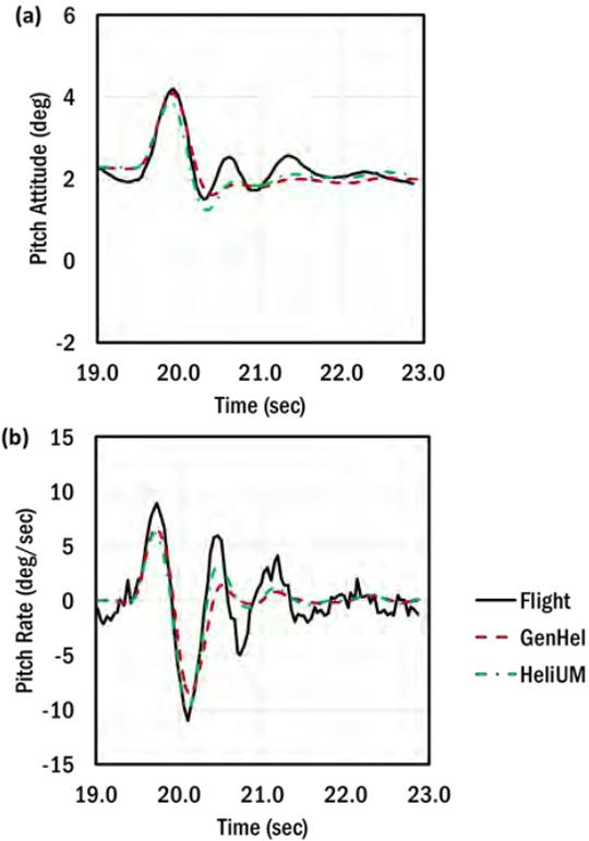
**Figure 24: Body Dynamic Response to Pitch Doublet at 200 knots**
