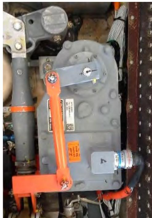
**Fig. 3: Collective trim servo on the AFDD EH-60L**
