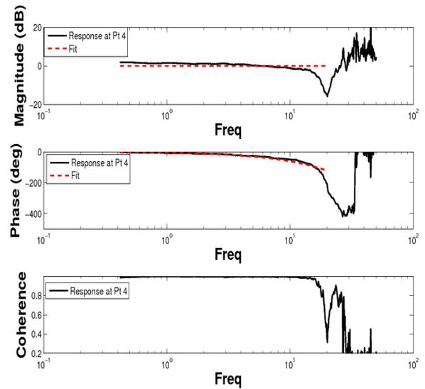
Figure 29: Frequency response of fitted rotor interference downwash at left horizontal stabilator (Point 4) as compared to the VPM prediction for a sweep of thrust
