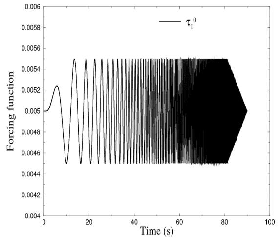
Figure 14: Sine sweep profile of rotor thrust based inflow forcing function at 80 knots
