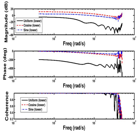
Figure 43: Frequency responses of the lower rotor inflow states as obtained from the lower rotor pitch moment sine sweep simulation
