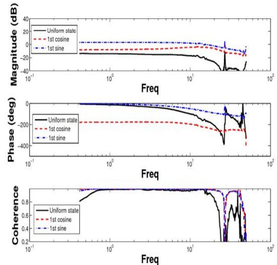
Figure 22: Frequency response of the rotor inflow states due to roll moment based inflow forcing function ( $\tau_2^{1s}$ ) excitation at 80 knots
