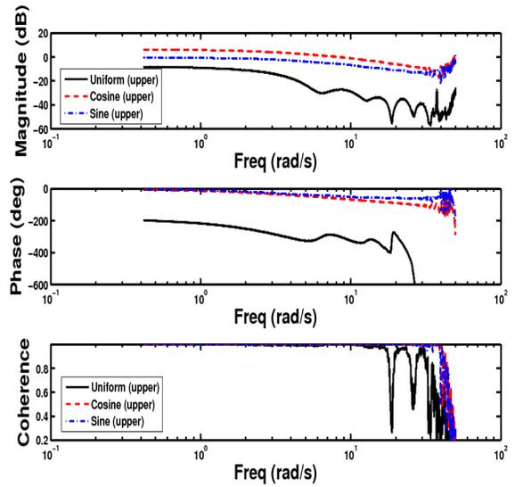
Figure 42: Frequency responses of the upper rotor inflow expansion coefficients as obtained from the lower rotor pitch moment sine sweep simulation
