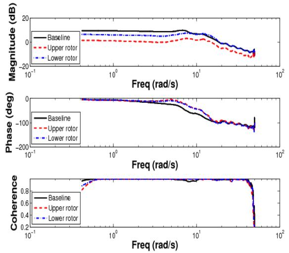
Figure 36: Frequency responses of the upper rotor uniform inflow expansion coefficient ( $\tilde{\alpha}_1^{01}$ ) and the lower rotor uniform inflow state ( $\alpha_1^{02}$ ) as obtained from the lower rotor thrust sine sweep simulation, along with the frequency response of baseline rotor uniform inflow state
