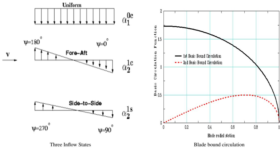
Figure 1: Illustration of 3 inflow states and basic blade bound circulation functions
