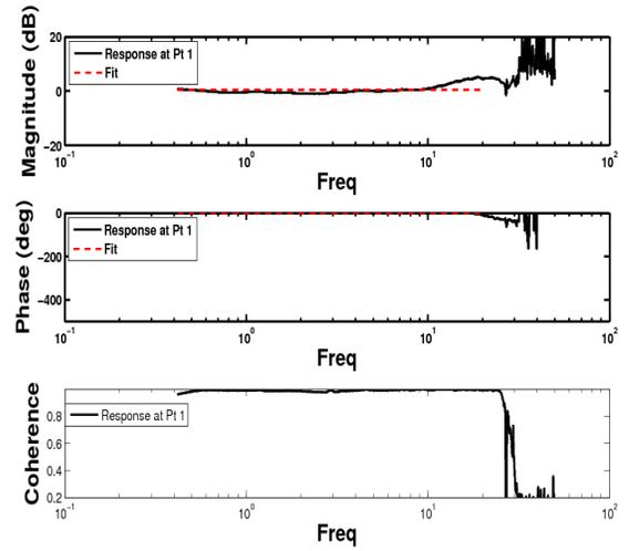
Figure 25: Frequency response of fitted rotor interference downwash at fuselage (Point 1) as compared to the VPM prediction for a sweep of thrust
