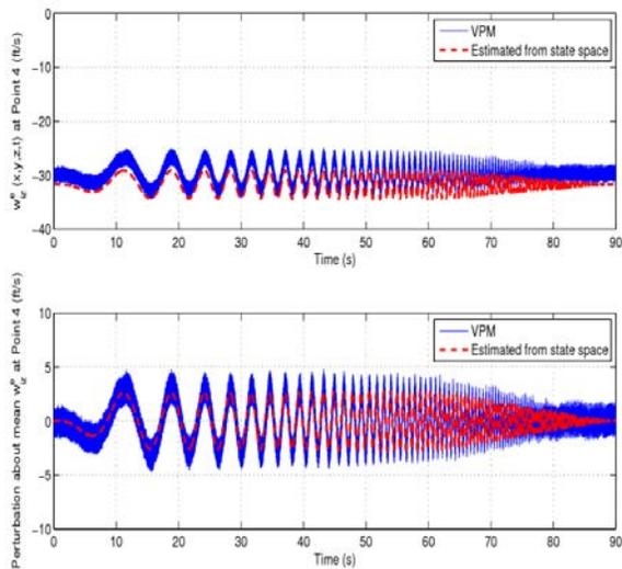
Figure 28: Time variation of fitted rotor interference downwash at left horizontal stabilator (Point 4) as compared to the VPM prediction
