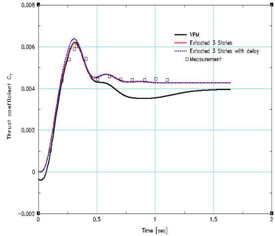
Figure 13: Rotor thrust coefficient response to the collective pull-up (48 deg/sec) in hover
