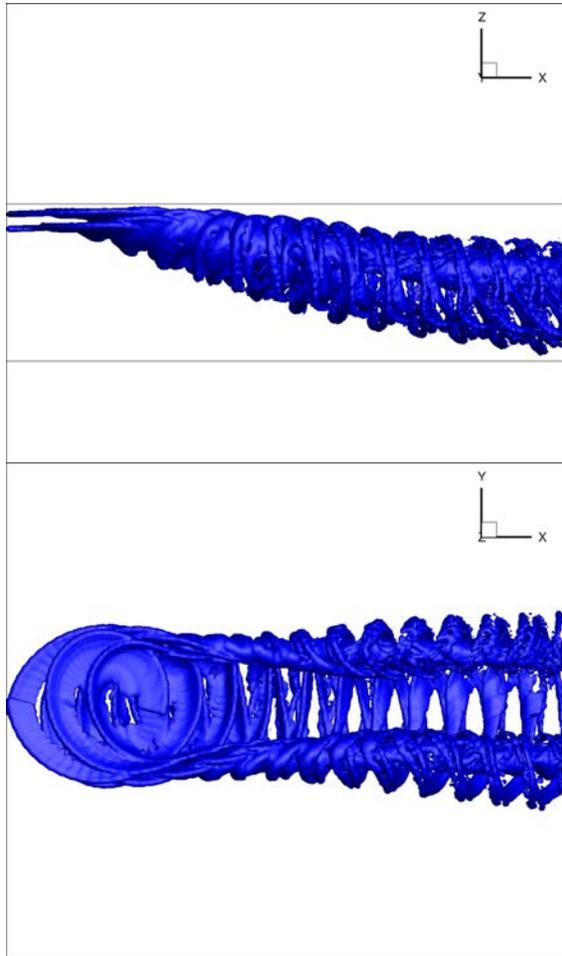
Figure 46: Side and top views of the rotor wake in steady state as obtained from a VPM simulation for a coaxial Harrington Rotor I in 40 knots forward flight
