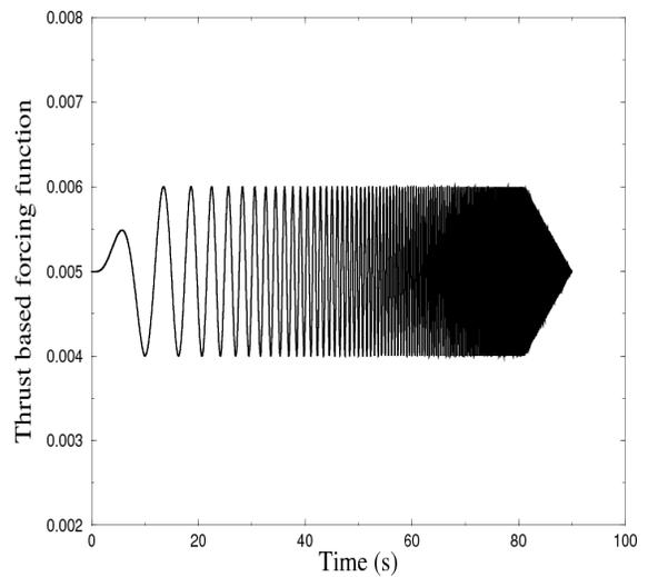
Figure 30: Time variation of the thrust based sine sweep forcing  $\tau_1^0$
