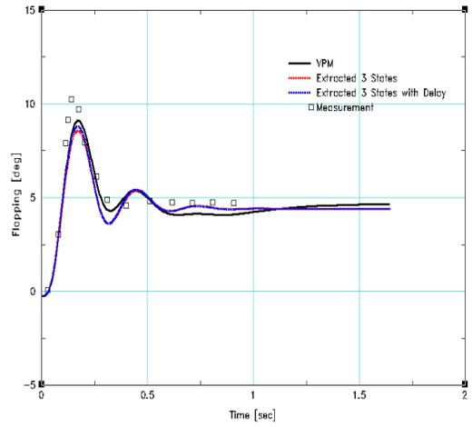
Figure 9: Rotor flapping (coning) response to the collective pull-up (200 deg/sec) in hover
