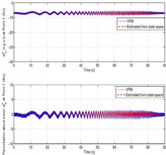
Figure 24: Time variation of fitted rotor interference downwash at fuselage (Point 1) as compared to the VPM prediction
