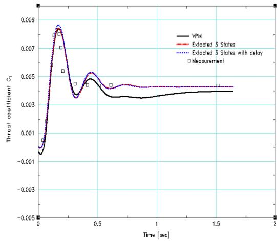
Figure 10: Rotor thrust coefficient response to the collective pull-up (200 deg/sec) in hover
