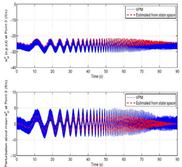
Figure 26: Time variation of fitted rotor interference downwash at vertical fin (Point 3) as compared to the VPM prediction
