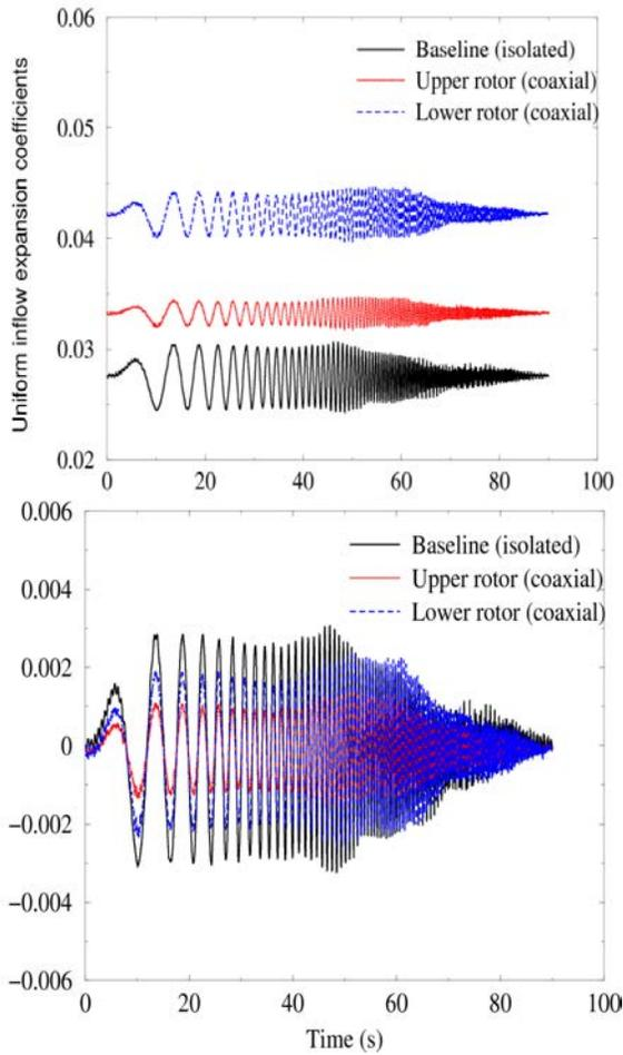
Figure 35: Time histories of the upper rotor uniform inflow expansion coefficient ( $\tilde{\alpha}_1^{01}$ ) and lower rotor uniform inflow state ( $\alpha_1^{02}$ ) as obtained from the lower rotor thrust sine sweep simulation, along with the baseline rotor uniform inflow state variation
