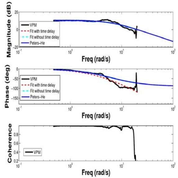
Figure 5: Frequency response of uniform inflow state to the thrust based forcing function ( $\tau_1^0$ ) in hover
