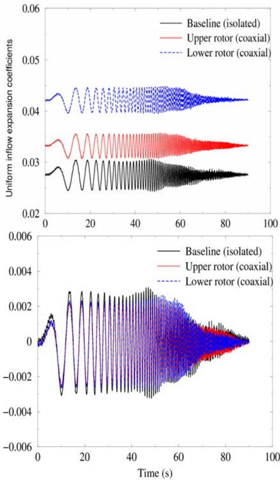
Figure 33: The time histories of the upper rotor uniform inflow state and the lower rotor uniform interference inflow expansion coefficient as obtained from the upper rotor thrust sine sweep simulation, along with the time history of the baseline rotor uniform inflow state
