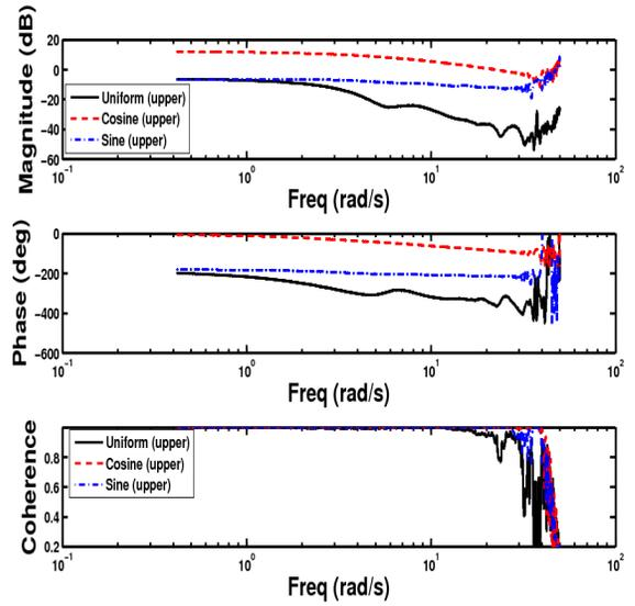
Figure 39: Frequency responses of the upper rotor inflow states as obtained from the upper rotor pitch moment sine sweep simulation ( $\tau_2^{1c1}$ ) in hover
