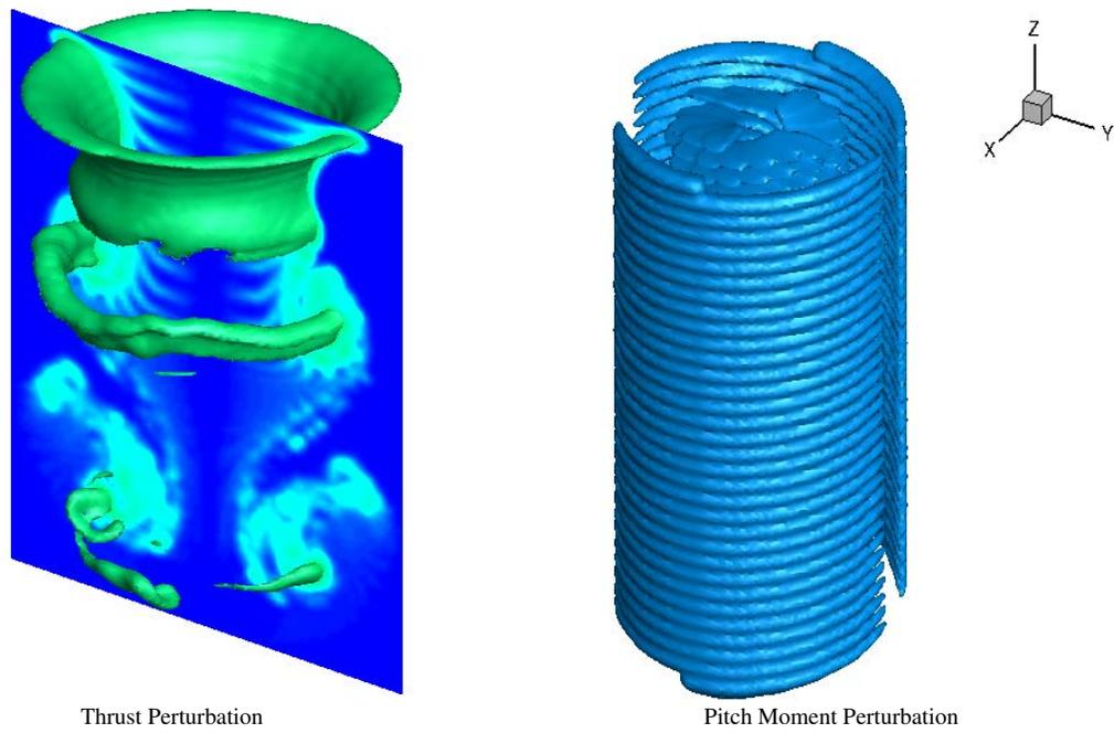
Figure 2: Rotor wake corresponding to the thrust and pitch moment perturbation in hover
