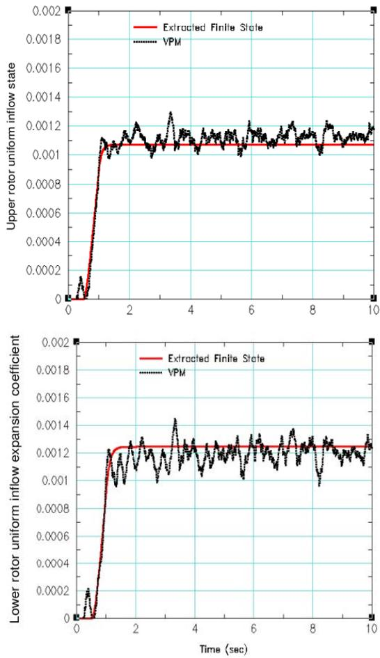
Figure 44: Upper rotor uniform inflow state and lower rotor uniform interference inflow expansion coefficients obtained as responses to a step ramp-up (0.5 sec) of thrust based inflow forcing function on the upper rotor
