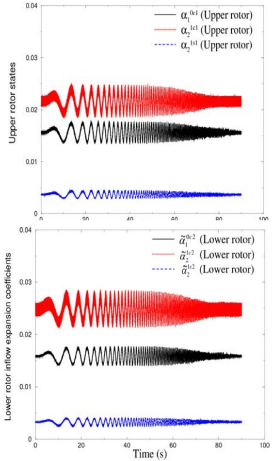
Figure 47: The upper rotor inflow states and the lower rotor interference inflow expansion coefficients as obtained from the VPM simulation with thrust sine sweep forcing applied to the upper rotor in forward flight at 40 knots
