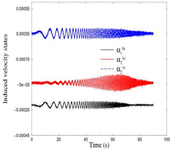
Figure 19: Rotor inflow states resulting from pitch moment based inflow forcing function ( $\tau_2^{1c}$ ) excitation at 80 knots
