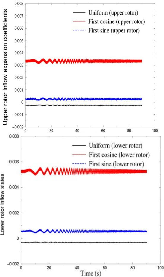
Figure 41: Upper rotor inflow expansion coefficients and the lower rotor inflow states as obtained from the lower rotor pitch moment sine sweep forcing
