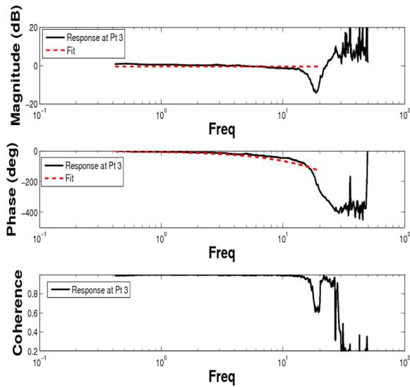
Figure 27: Frequency response of fitted rotor interference downwash at vertical fin (Point 3) as compared to the VPM prediction for a sweep of thrust
