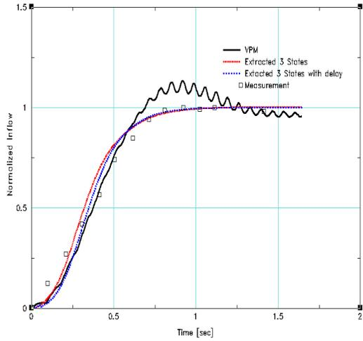
Figure 11: Rotor inflow response to the collective pull-up (48 deg/sec) in hover
