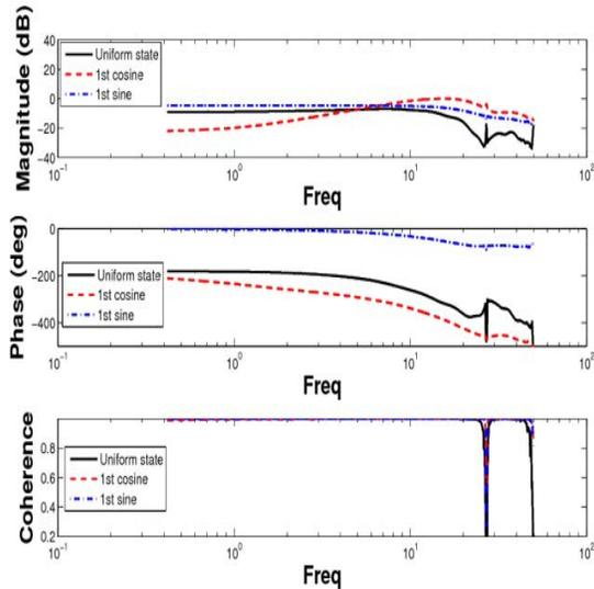
Figure 20: Frequency response of the rotor inflow states due to pitch moment based inflow forcing function ( $\tau_2^{1c}$ ) excitation at 80 knots
