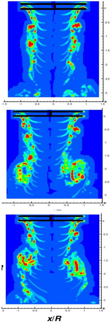
Figure 31: Comparison of the vorticity contours along the longitudinal plane passing through the rotor hub, as obtained in steady state, and at  $t = 90$  s for the thrust-based sine sweep forcing applied to the upper and the lower rotors
