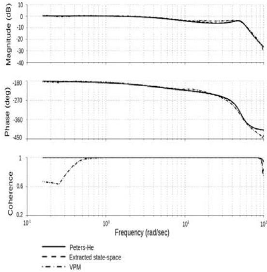
Figure 7: Frequency response of rotor longitudinal flapping to the cyclic pitch in hover
