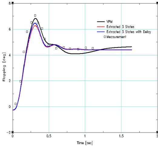
Figure 12: Rotor flapping (coning) response to the collective pull-up (48 deg/sec) in hover
