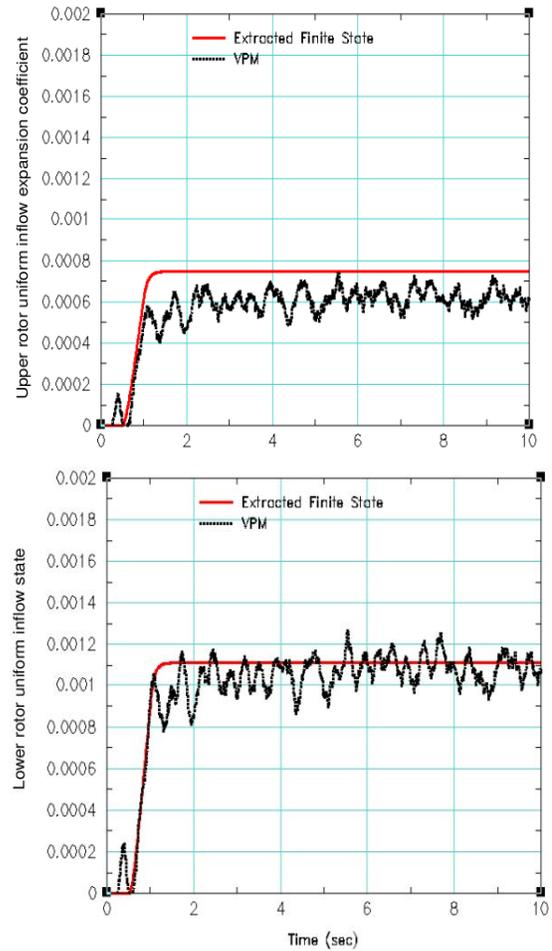
Figure 45: Upper rotor uniform inflow state and lower rotor uniform interference inflow expansion coefficient obtained as responses to a step ramp-up (0.5 sec) of thrust based inflow forcing function on the lower rotor
