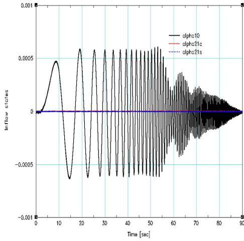
Figure 3: Inflow state response to the frequency sweep of thrust based inflow forcing function ( $\tau_1^0$ ) in hover
