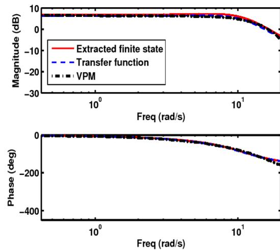
Figure 18: Comparison of frequency response of the cosine inflow state from state-space model, transfer function fit, and VPM simulation data due to thrust based excitation at 80 knots
