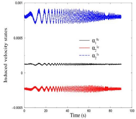
Figure 21: Rotor inflow states resulting from roll moment based inflow forcing function ( $\tau_2^{1s}$ ) excitation at 80 knots
