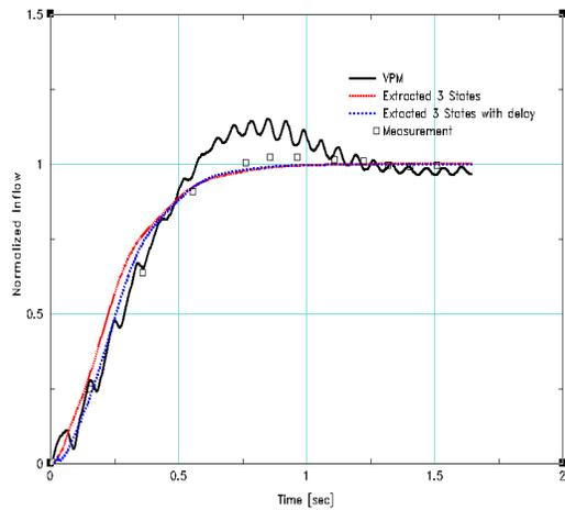
Figure 8: Rotor inflow response to the collective pull-up (200 deg/sec) in hover
