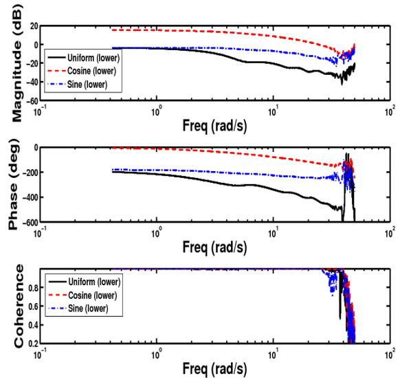
Figure 40: Frequency responses of the lower rotor inflow expansion coefficients as obtained from the upper rotor pitch moment sine sweep simulation ( $\tau_2^{1c1}$ ) in hover
