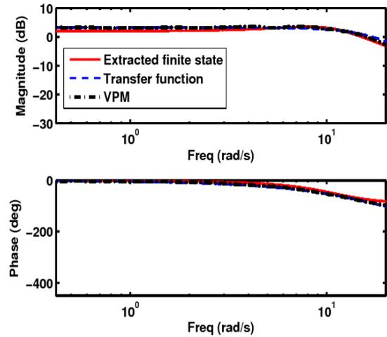
Figure 17: Comparison of frequency response of the uniform inflow state from state-space model, transfer function fit, and VPM simulation data due to thrust based excitation at 80 knots
