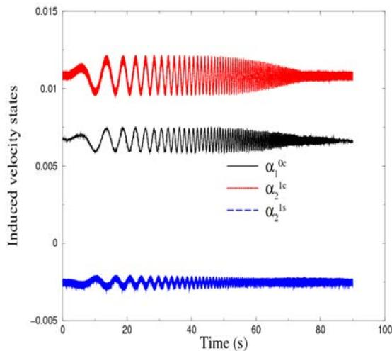
Figure 16: Rotor inflow states resulting from thrust based inflow forcing function excitation at 80 knots
