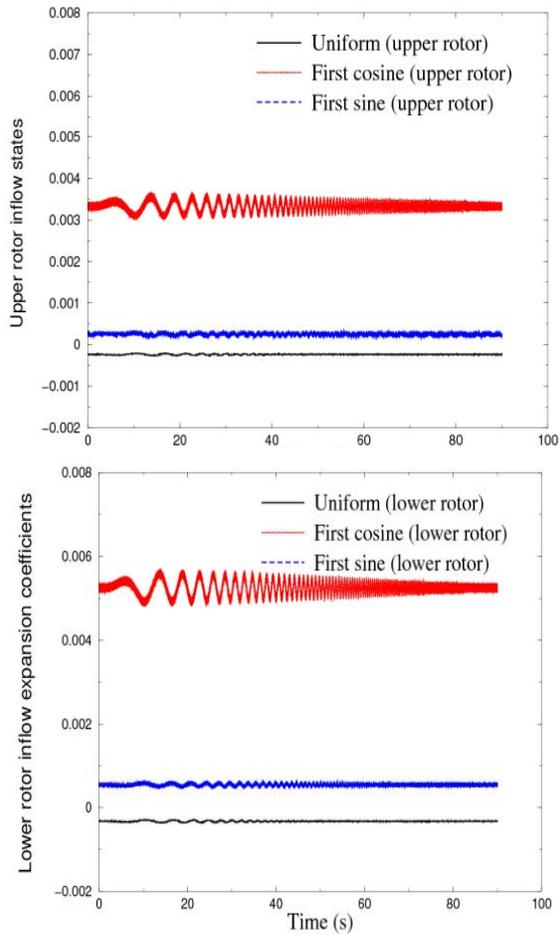
Figure 38: Upper rotor inflow states and the lower rotor interference expansion coefficients as obtained from the upper rotor pitch moment based sine sweep forcing in hover
