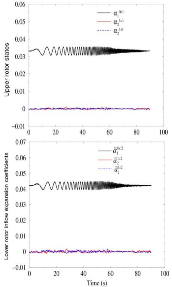
Figure 32: Upper rotor inflow states and lower rotor interference inflow expansion coefficients as obtained from the VPM simulation with the thrust sine sweep forcing  $\tau_1^{01}$  applied to the upper rotor
