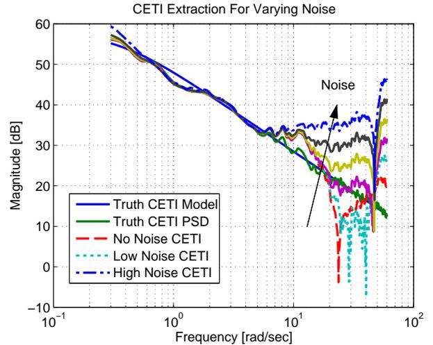
**Fig. 13. Extracted CETI models with varying measurement noise**
