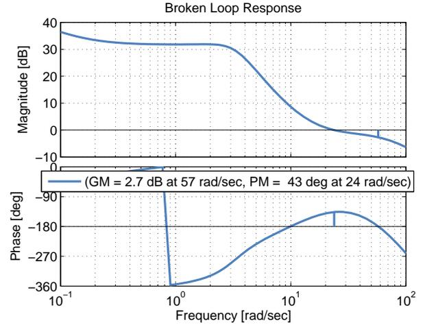
Fig. 5. Simulation broken loop response
