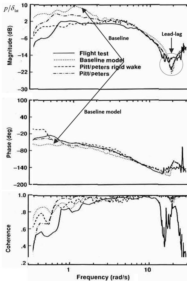
(b) UH-60 blade element model correlation with system identification flight-test data ( $p/\delta_{lat}$ , hover)
