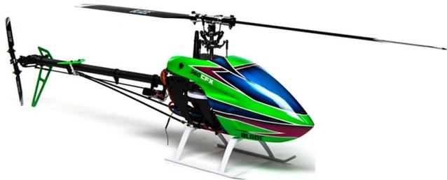
(a) 360CFX flybarless helicopter UAV (rotor diameter = 0.81 m)
