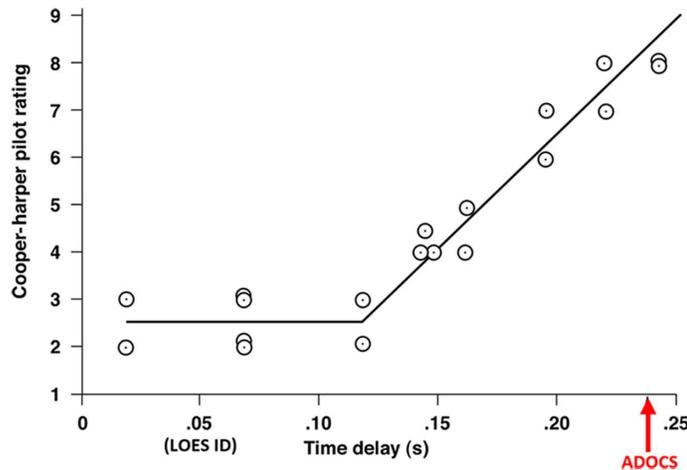
(a) Extensive fixed-wing flight-test studies on the importance of time delay to handling qualities, F-8, NT-33 (Ref. 16)
