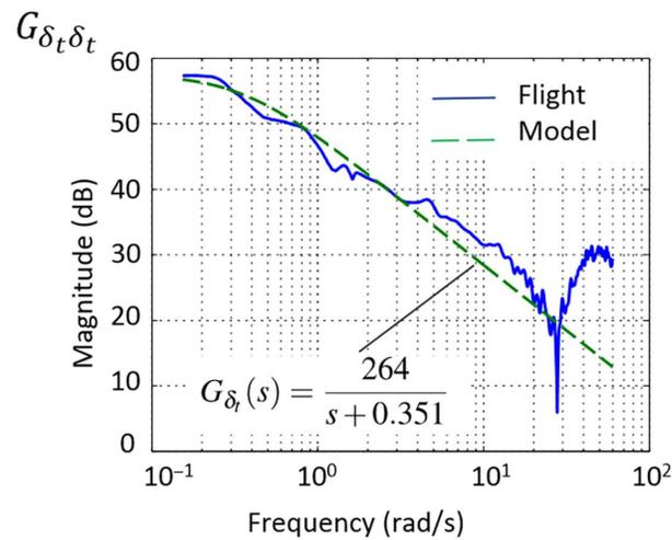
(b) Longitudinal CETI turbulence identification from flight (Ref. 110)
