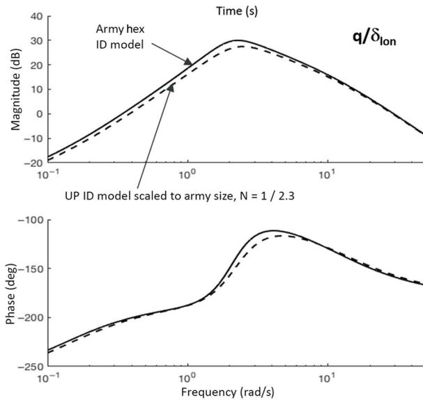
(c) Excellent agreement of froude-scaled dynamics of small-scale and larger-scale hexicopter ID with dynamics based on hub-to-hub scaling
