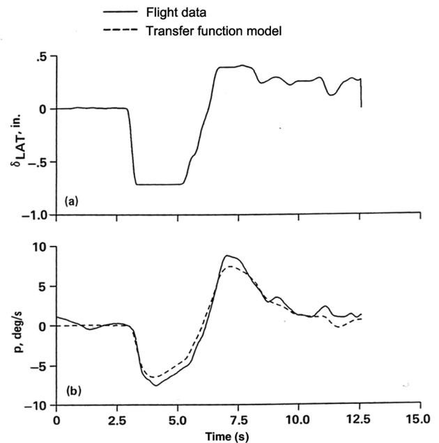
(d) Good agreement of time response of identified lowerorder transfer function model with flight data
