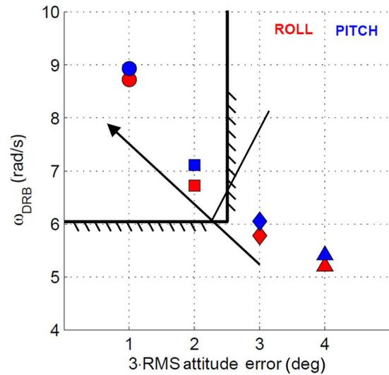
(d) Close correlation of DRB requirements with turbulence performance in flight (Ref. 111)
