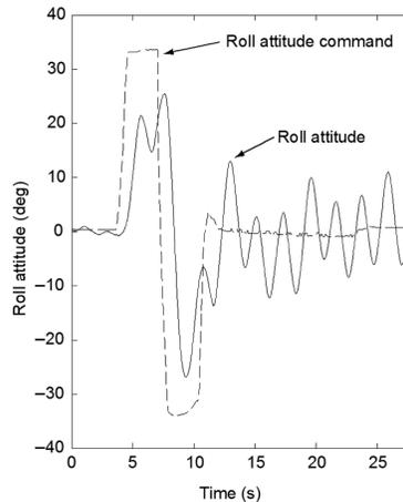
(b) Roll response for initial FCS design based on estimated delay
