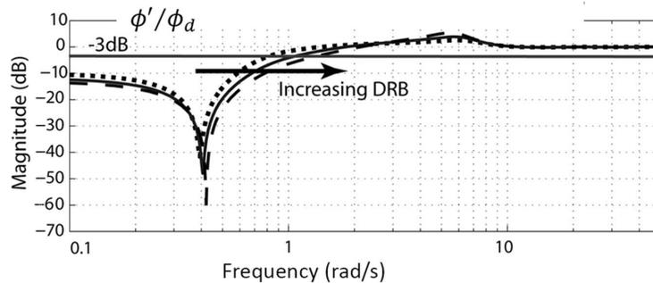
(b) Determination of roll DRB for three different control system configurations (JUH-60A RASCAL flight test) criteria
