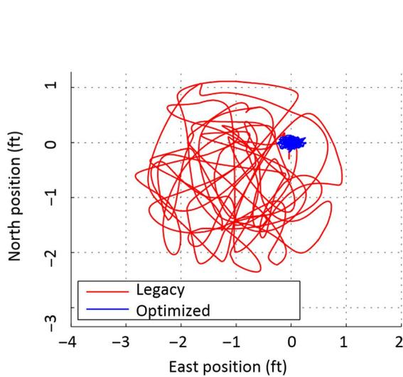
(c) Large flight-test improvement of optimized control system over legacy system (Ref. 111)
