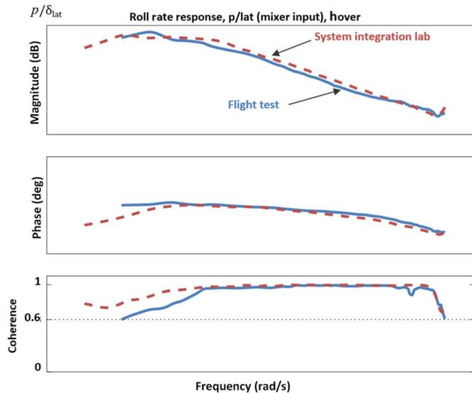
(b) Comparison of System Integration Lab (SIL) model and flight-test data for roll response in hover;  $p/\delta_{lat}$
