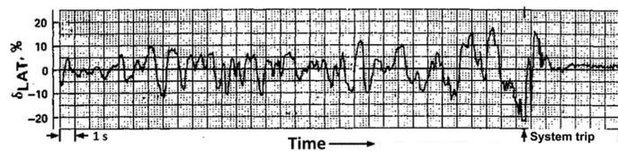
(b) ADOCS - 1 Hz PIO in slope landing (high-gain task) (Ref. 17)
