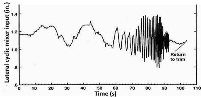
(a) Piloted flight-test frequency sweep input  $\delta_{lat}$  in hovering flight (UH-60)
