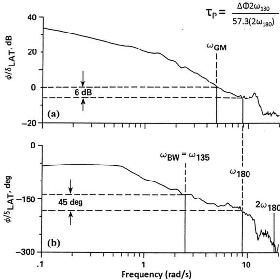
Fig. 7. ADS-33 metrics were obtained from frequency response identification of B214ST (Ref. 14).
