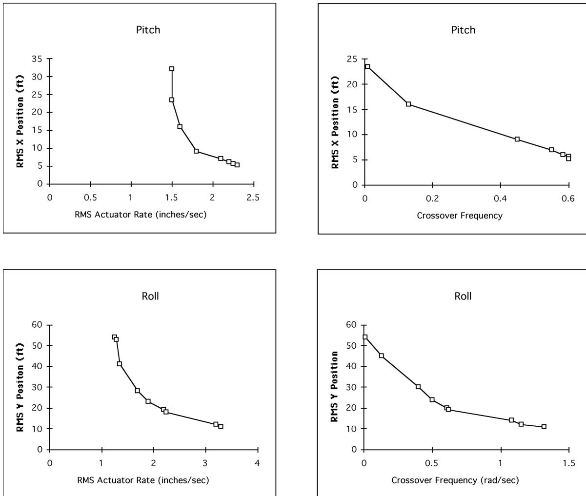
Fig. 16 CONDUIT studies showing trade-off of position station accuracy against required actuator rate and crossover frequency.
