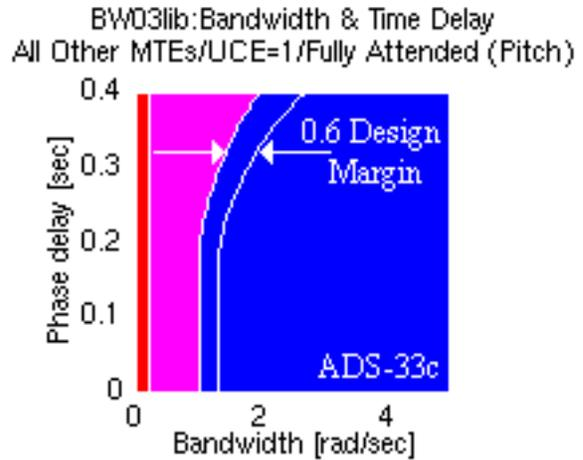
Fig. 4 Bandwidth specification including a 0.6 design margin.
