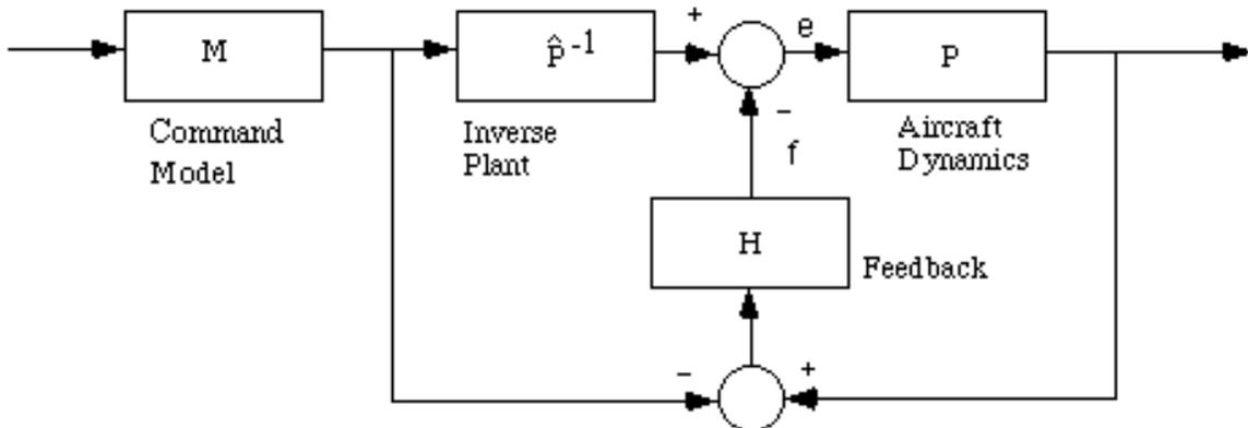
Fig. 11 Model-following block diagram.
