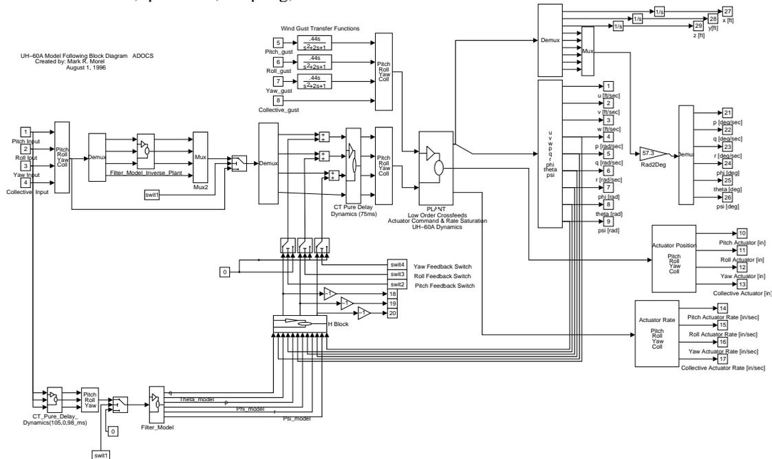
Fig. 12 SIMULINK diagram of the RASCAL model-following control laws.
