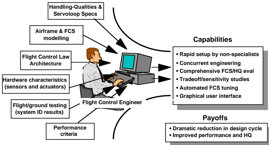
Fig. 1 CONDUIT control system integration and design evaluation process.
