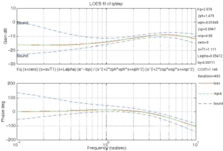
Fig. 26 Optimized X-29A LOES parameters.
