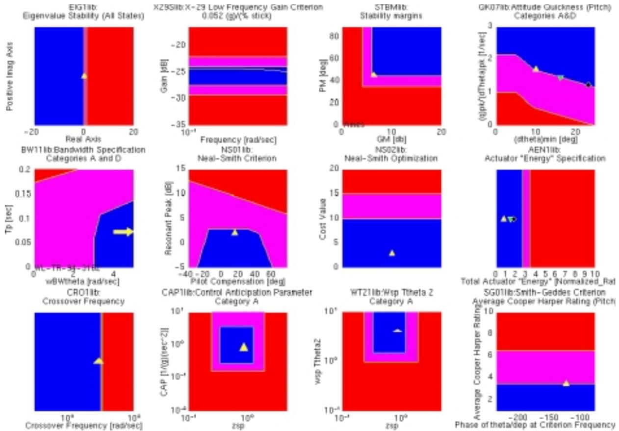
Fig. 21 Optimized X-29A performance and handling qualities results (with quickness filter).
