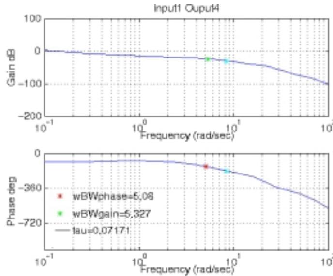
Fig. 24 Optimized X-29A bandwidth requirement results.
