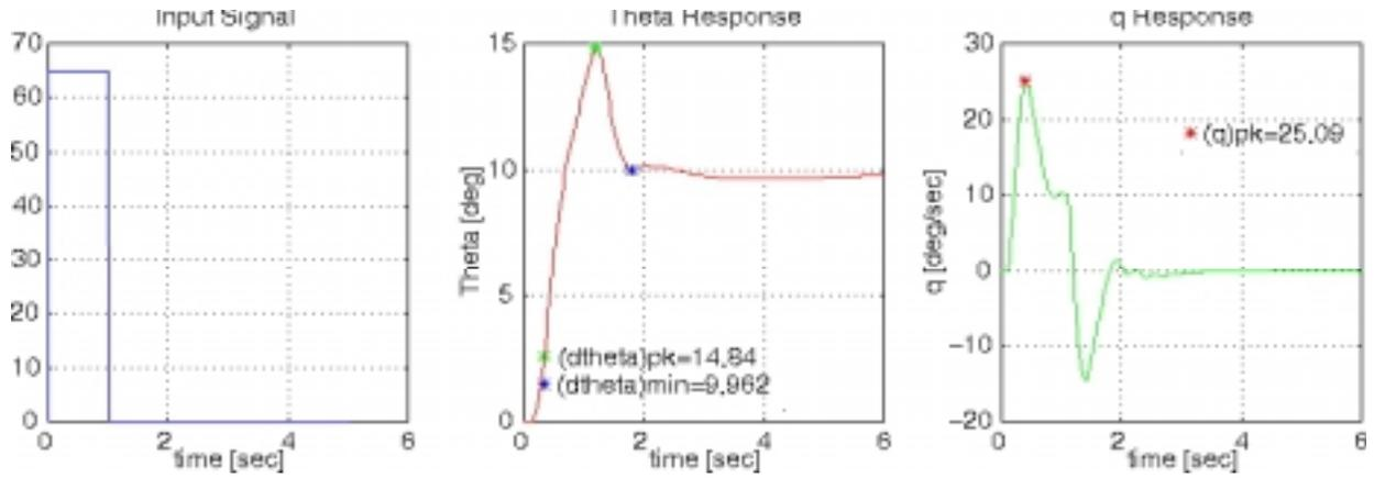
Fig. 23 Optimized X-29A moderate amplitude quickness requirement results.
