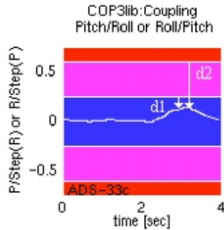
Fig. 7 Specifications that use vector data have the value determined by the “worst point” of the vector.
