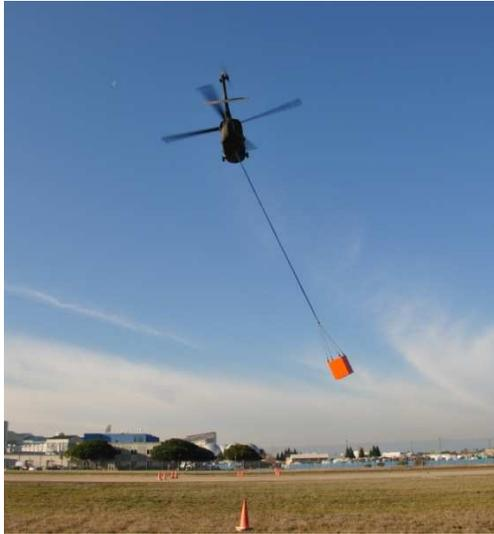
Figure 1. UH-60 with external load.
