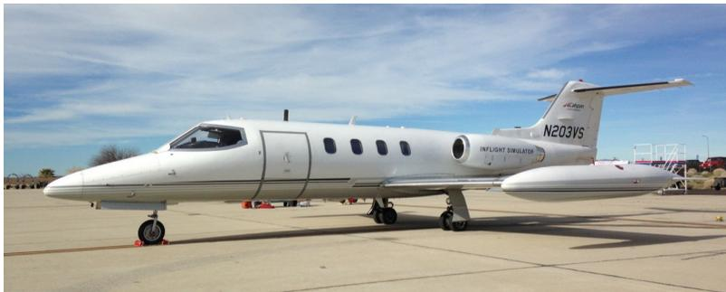
Figure 3. Calspan Variable Stability System Learjet LJ-25D.
