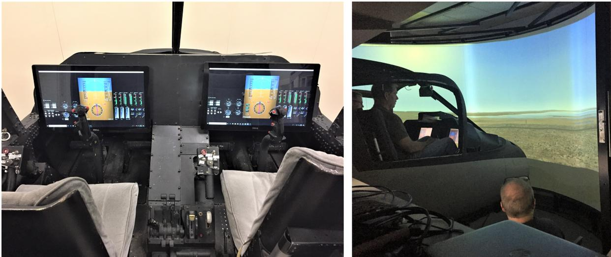
Figure 15. Cockpit inceptors and displays (left) and flight simulation facility (right).
