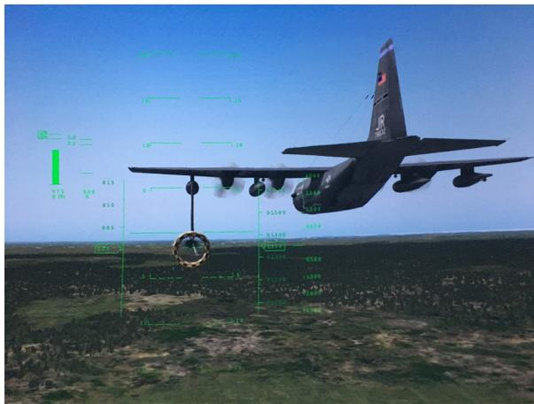
Fig. 16. Pilot's view of formation position (note waterline symbol over refueling basket).
