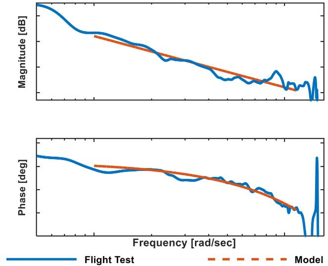
**Figure 13. Lateral Cyclic to roll rate frequency response from JIO and low order transfer function approximation.**
