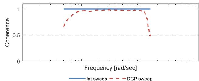
**Figure 6. Lateral cyclic to DCP coherence is close to 1 for the entire frequency range, indicating complete cross-control correlation between the effectors.**
