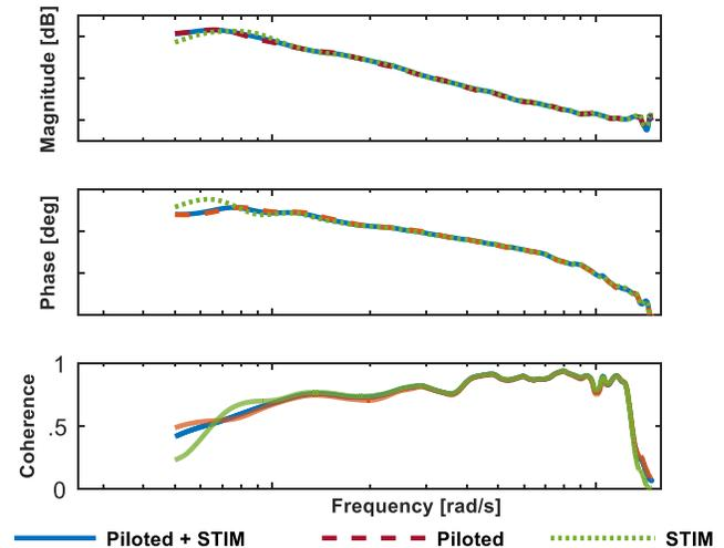
**Figure 8. Roll rate due to DCP frequency response for automated versus piloted frequency sweeps.**
