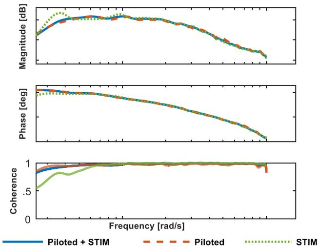
**Figure 7. Roll rate due to lateral stick (closed-loop) frequency response for automated versus piloted frequency sweeps.**
