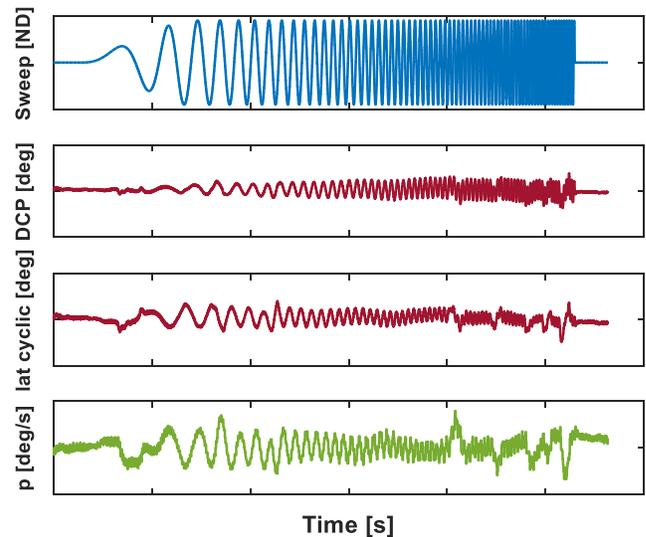
**Figure 5. Automated DCP effector sweep in hover shows that DCP and Lateral Cyclic (at the rotor head) are highly-correlated.**
