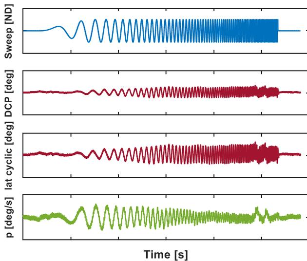
**Figure 4. Automated lateral stick sweep in hover shows that DCP and Lateral Cyclic (at the rotor head) are highly-correlated.**
