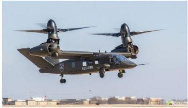
**Figure 1. V-280 in VTOL Mode flight.**
