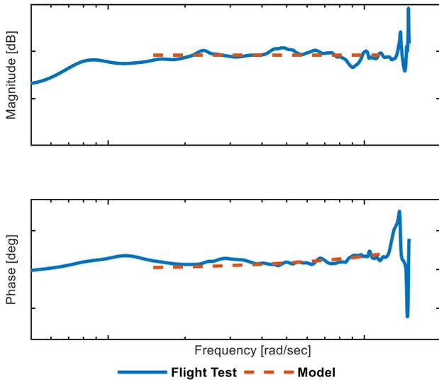
**Figure 14. Ratio of p/DCP and p/(lateral cyclic) frequency response from JIO and transfer function approximation.**
