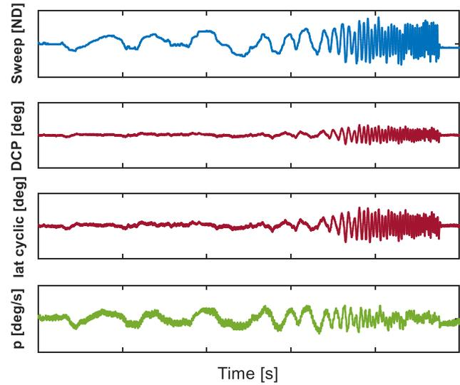
**Figure 3. Piloted lateral stick sweep in hover shows that DCP and Lateral Cyclic (at the rotor head) are highly-correlated.**
