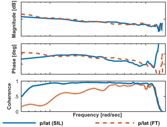
**Figure 11. Flight Test and SIL comparison of Lateral Cyclic to roll rate frequency response.**
