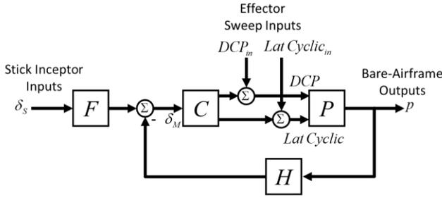
**Figure 2. Top level V-280 closed-loop block diagram (lateral axis, hover).**
