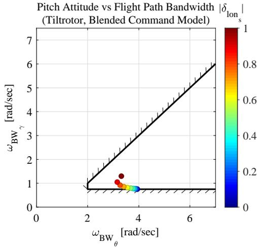
**Fig. 19. Flight path versus pitch attitude bandwidth values for fight path rate blended command model (tiltrotor).**
