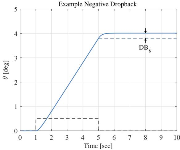
**Fig. 7. Example pitch attitude step response time history showing definition of negative pitch attitude dropback  $DB_{\theta}$ .**
