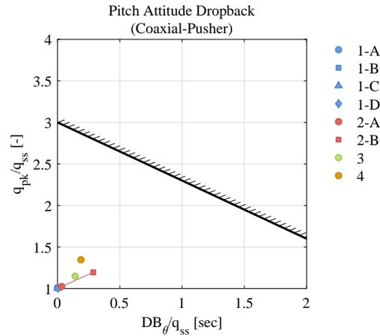
**Fig. 11. Pitch attitude dropback values for command model variations (coaxial-pusher).**
