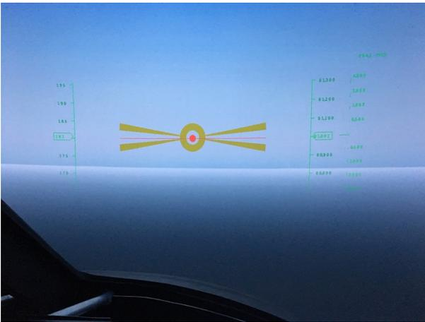
**Fig. 22. Display for Pitch Sum-of-Sines Tracking and Attitude Capture and Hold tasks.**
