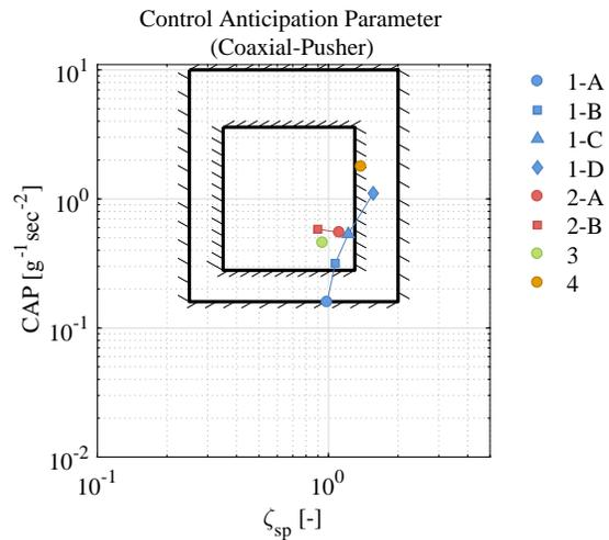
**Fig. 12. Control anticipation parameters values for command model variations (coaxial-pusher).**
