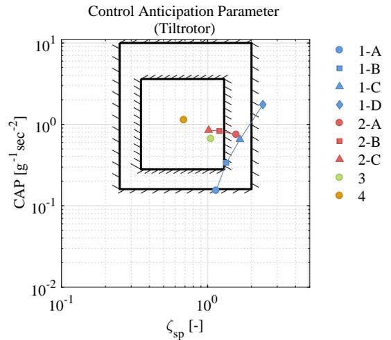
**Fig. 17. Control anticipation parameters values for command model variations (tiltrotor).**
