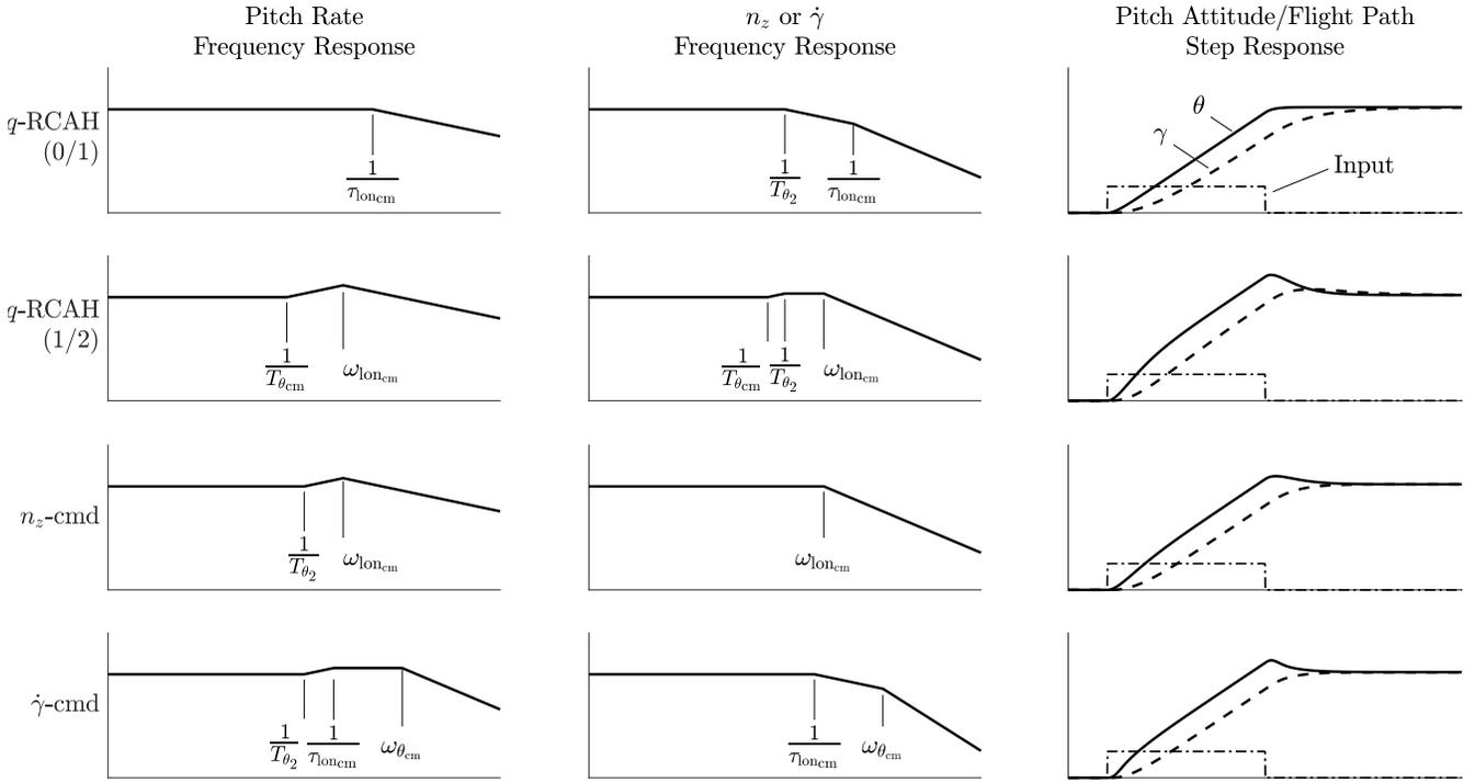
**Fig. 6. Characteristics of pitch axis response types.**
