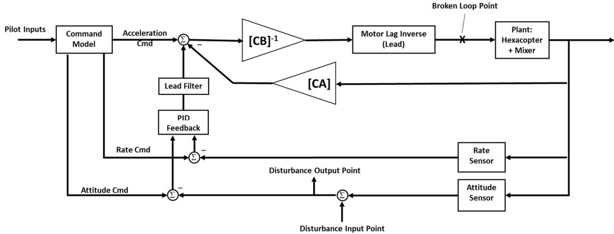
Figure 4. Inner-loop dynamic inverse with PID control for attitude command.
