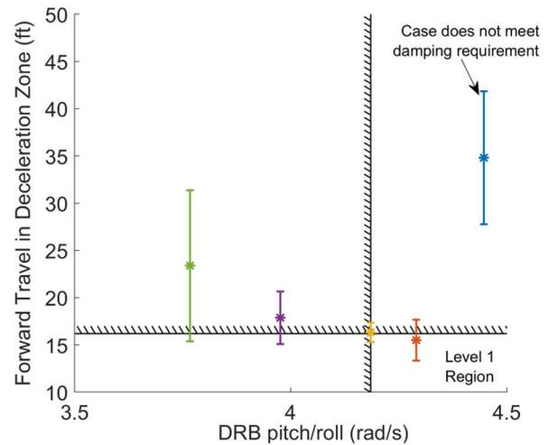
Figure 10. Emergency stop tracking performance versus DRB from flight test.
