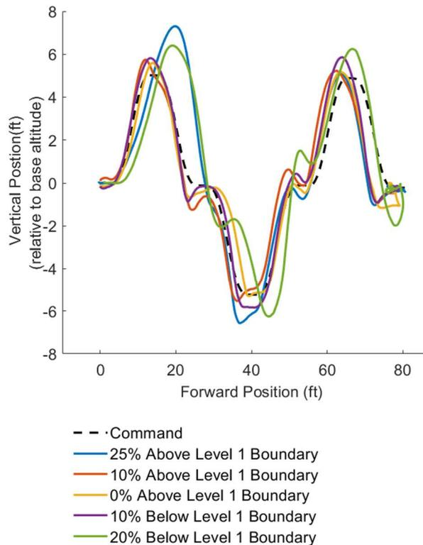
Figure 7. Object avoidance example flight test data.
