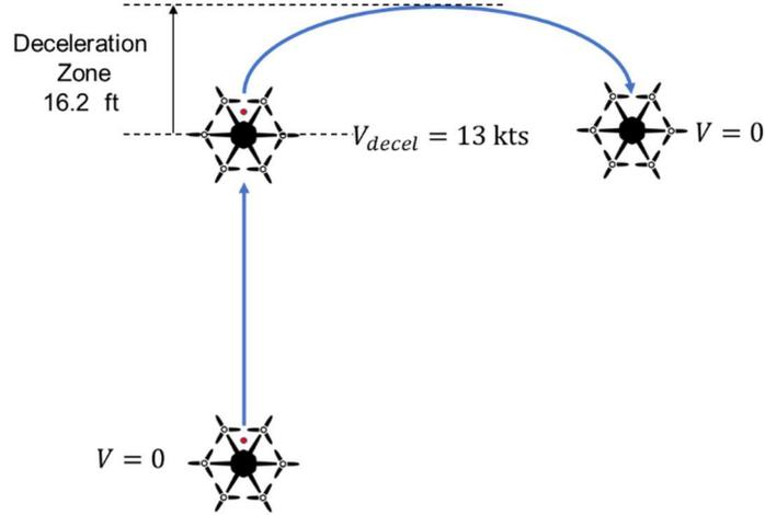
Figure 2. Emergency stop course for the UP Hexacopter, top view.
