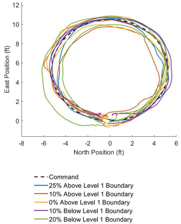
Figure 15. Pirouette example flight test data.
