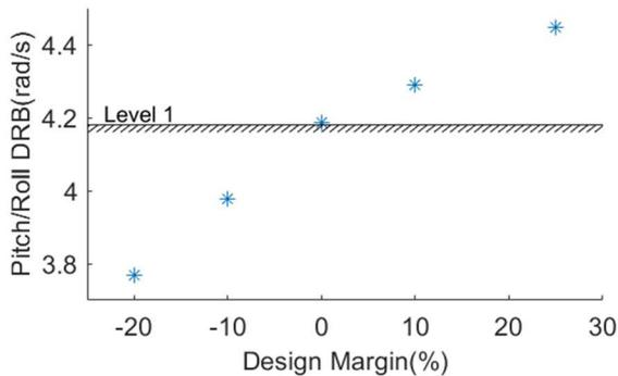
Figure 6. Flight test cases for UP hexacopter, pitch and roll DRB versus design margin.
