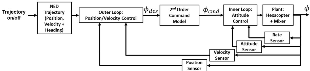
Figure 17. Closed-loop architecture of the UP hexacopter.
