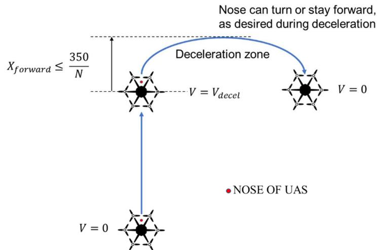
Figure 26. Course trajectory for emergency stop.
