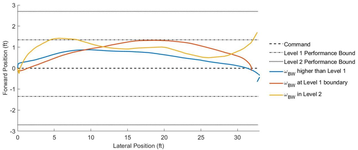
Figure 21. Lateral reposition example flight test data for attitude bandwidth flight tests on the Synergy 626.
