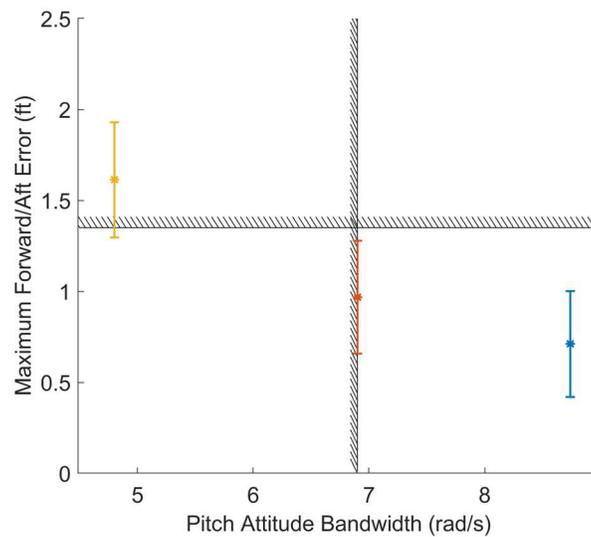
Figure 22. Lateral reposition performance versus attitude bandwidth from flight test on the Synergy 626.
