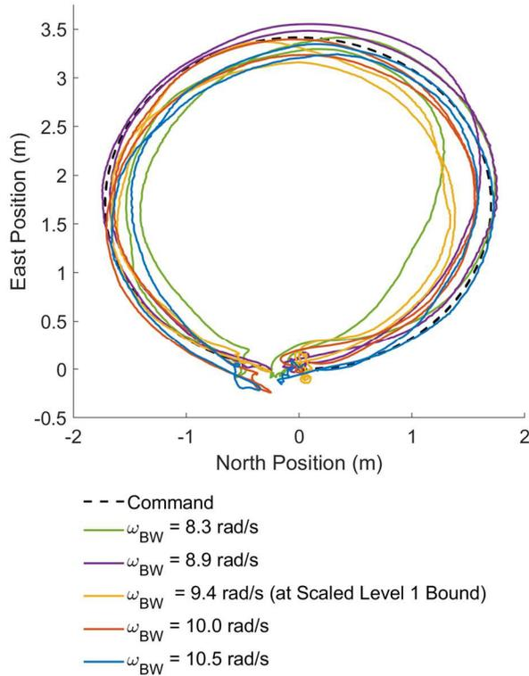
Figure 18. Pirouette example flight test data for attitude bandwidth flight tests.
