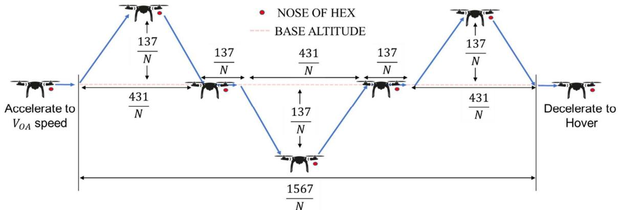
Figure 25. Course trajectory for object avoidance (dimensions are in feet).
