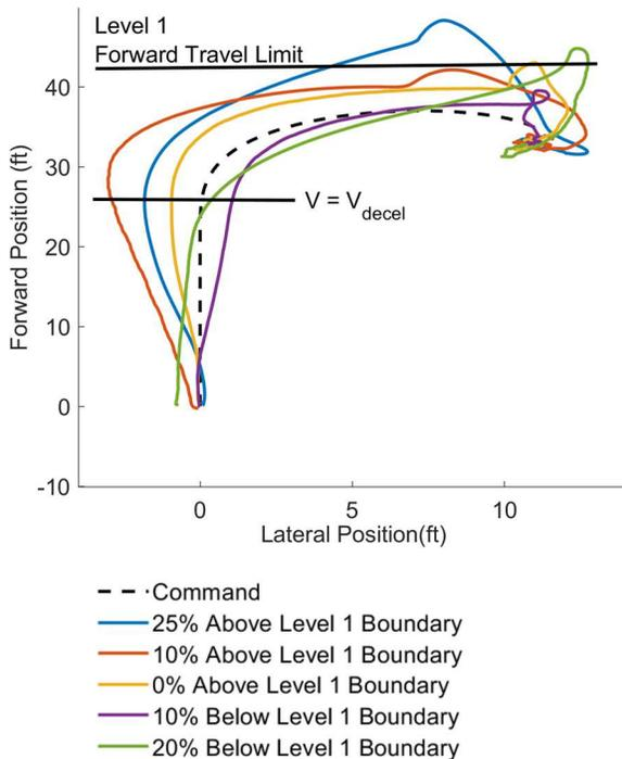
Figure 9. Emergency stop example flight test data.
