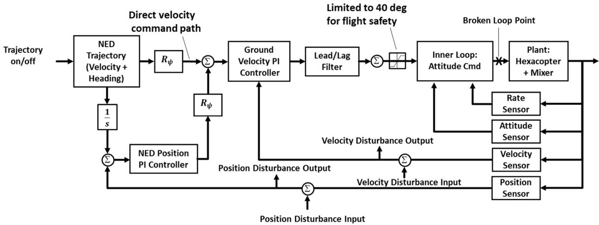
Figure 5. Outer-loop PI control for trajectory velocity and position tracking.
