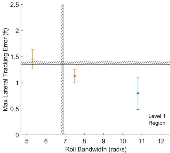
Figure 24. Depart/Abort performance versus attitude bandwidth from flight test on the Synergy 626.
