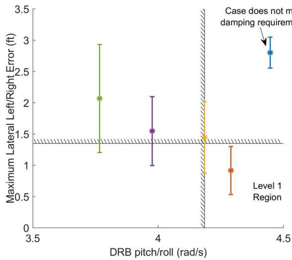
Figure 14. Depart/Abort tracking performance versus DRB from flight test.
