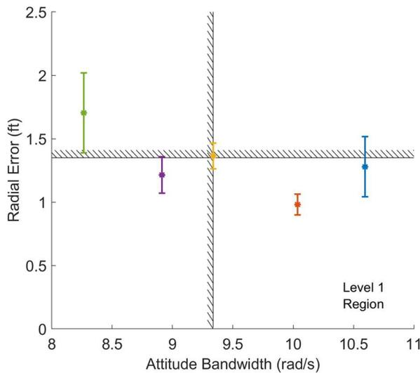
Figure 19. Pirouette tracking performance versus attitude bandwidth from flight test.
