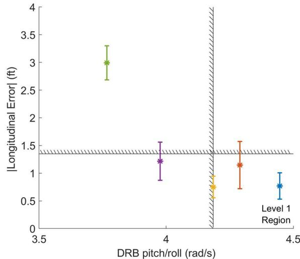
Figure 12. Lateral reposition tracking performance versus DRB from flight test.
