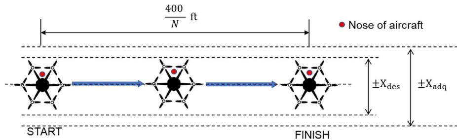
Figure 27. Course trajectory for lateral reposition.
