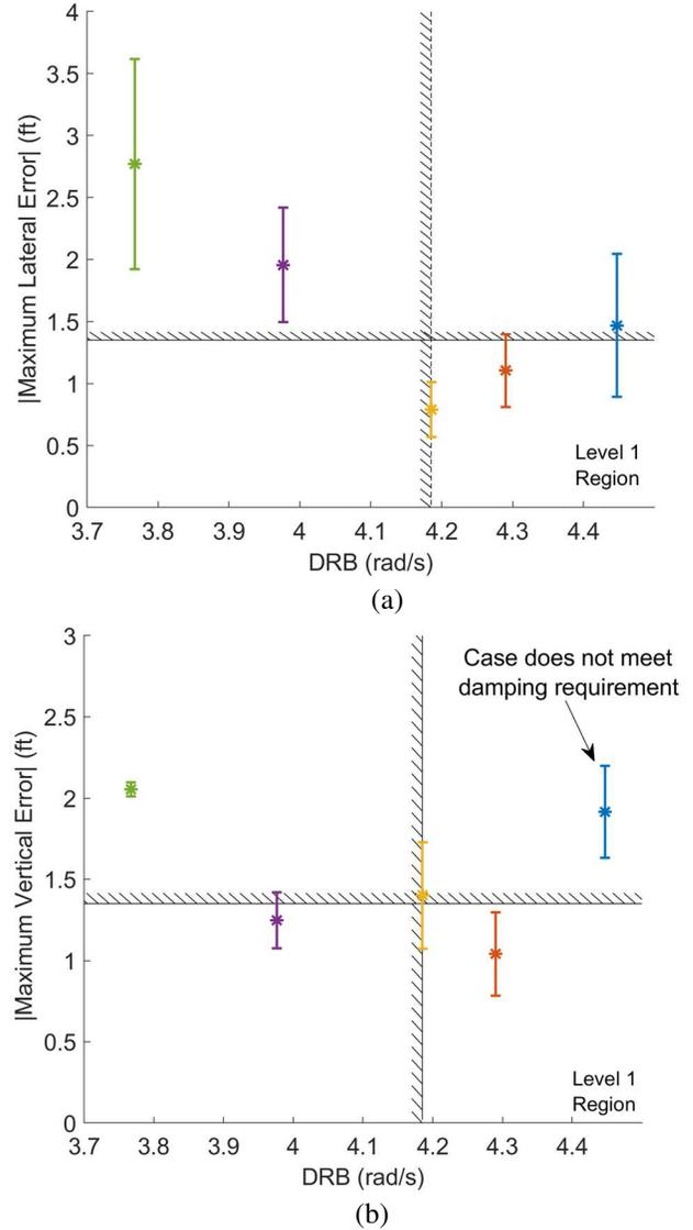
Figure 8. Object avoidance tracking performance versus DRB from flight test.
