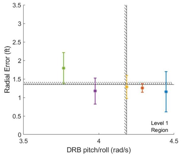
Figure 16. Pirouette tracking performance versus DRB from flight test.
