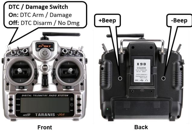
Fig. 19. The Taranis radio used in the Piasecki simulation environment and flight test.
