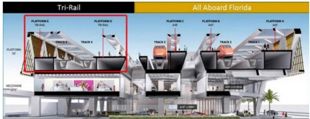
Figure 7.23 [137] shows how the Tri-Rail and the Brightline trains share tracks on the elevated platforms at the MiamiCentral Station. [138]
