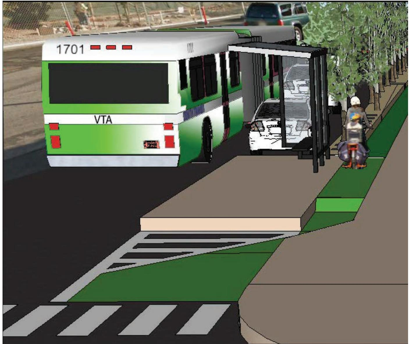
**Figure 8.2 - Separated Bike Lane.** Example of how a separated bike lane can coexist with a dedicated bus lane on a busy street. Image by Beth Martin of Fall 2014 Urban Design Studio, San José State University.
