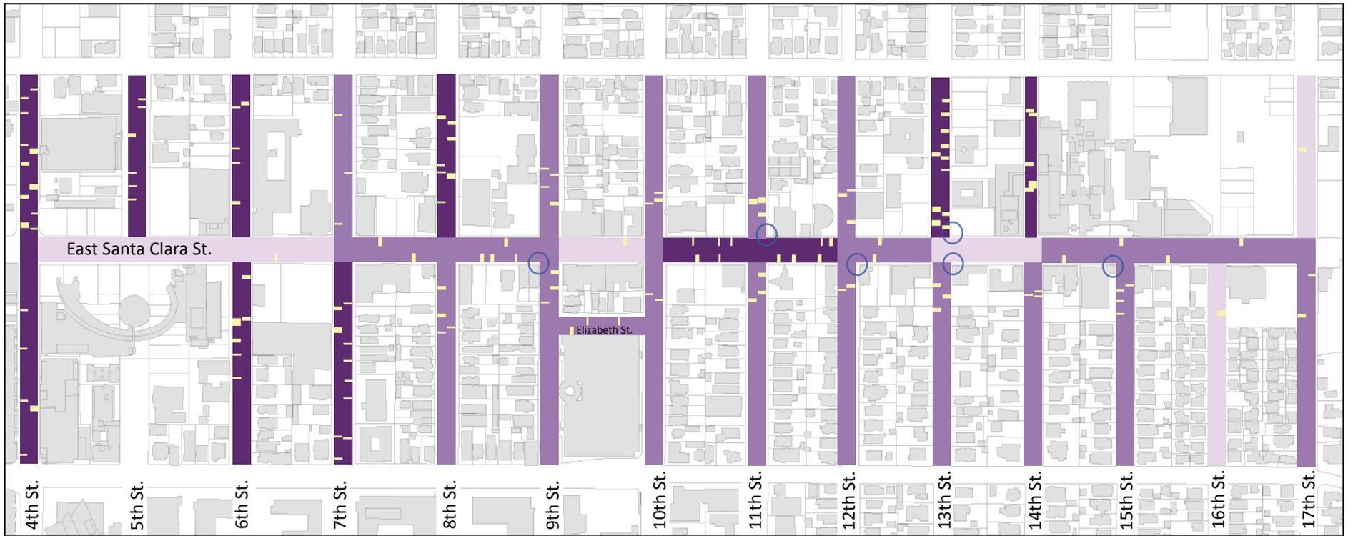
**Figure 4.17 Curb Cut Locations & Sidewalk Ramp Conditions Along East Santa Clara Street** 0 125 250 500 Feet
