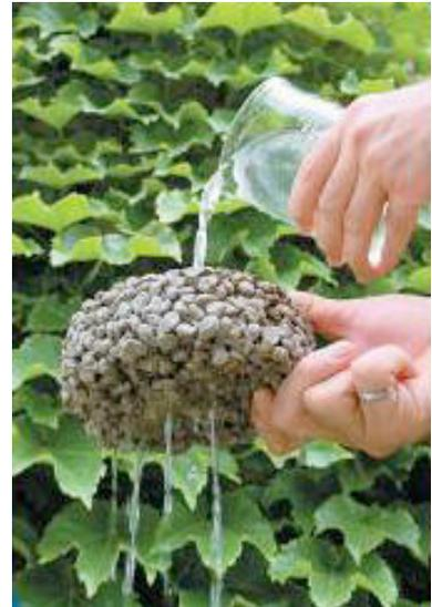
**Figure 10: Pervious Concrete**
