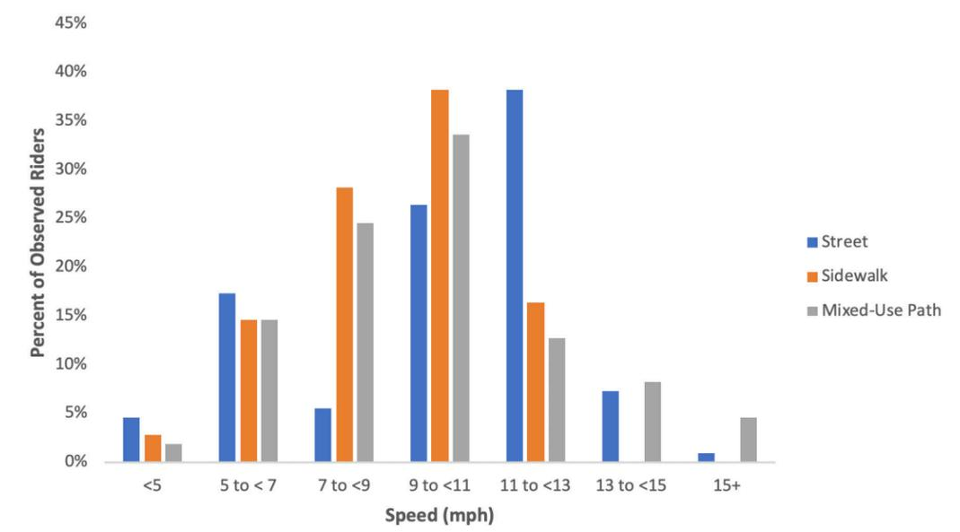
FIGURE 16. DISTRIBUTION OF E-SCOOTER RIDER SPEEDS ON DIFFERENT TYPES OF TRANSPORTATION FACILITIES.
