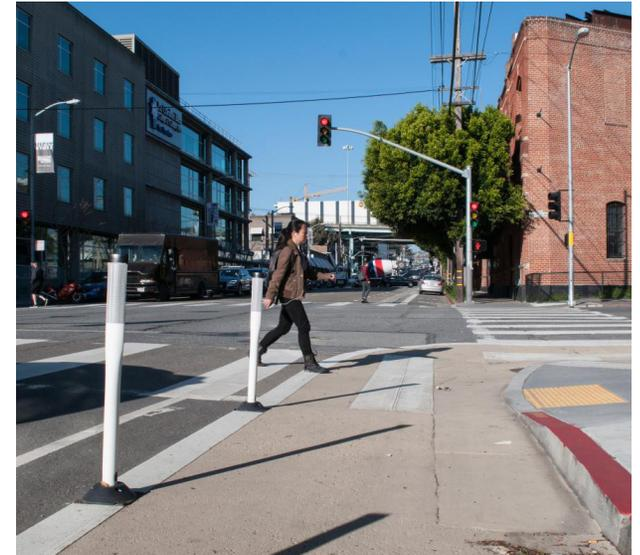
Soft hit posts and contrasting tan paint daylight the intersection. Daylighting treatments are added to intersections to increase visibility for both pedestrians and motorists.
