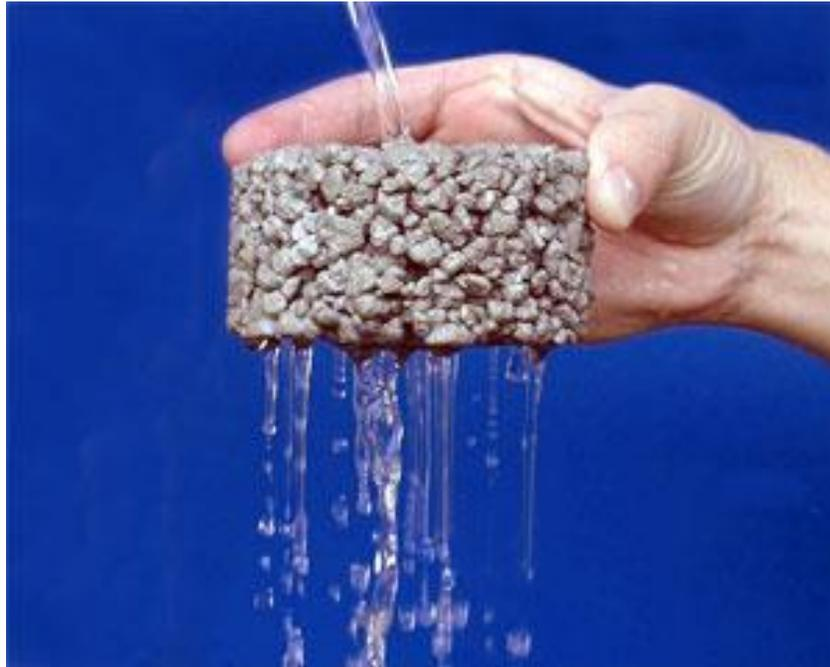
FIGURE 4 PERMEABLE PAVEMENT
